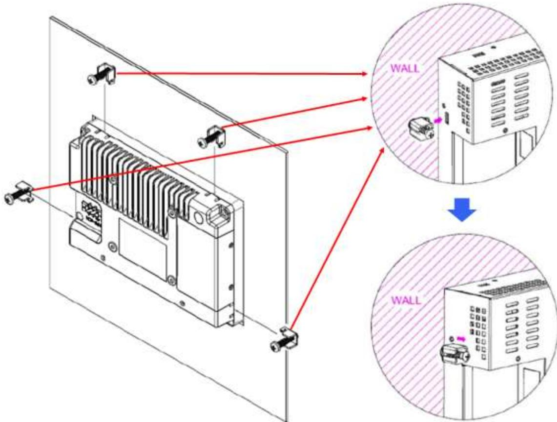
**Figure 2.1: Panel Mounting of FABS Series**
