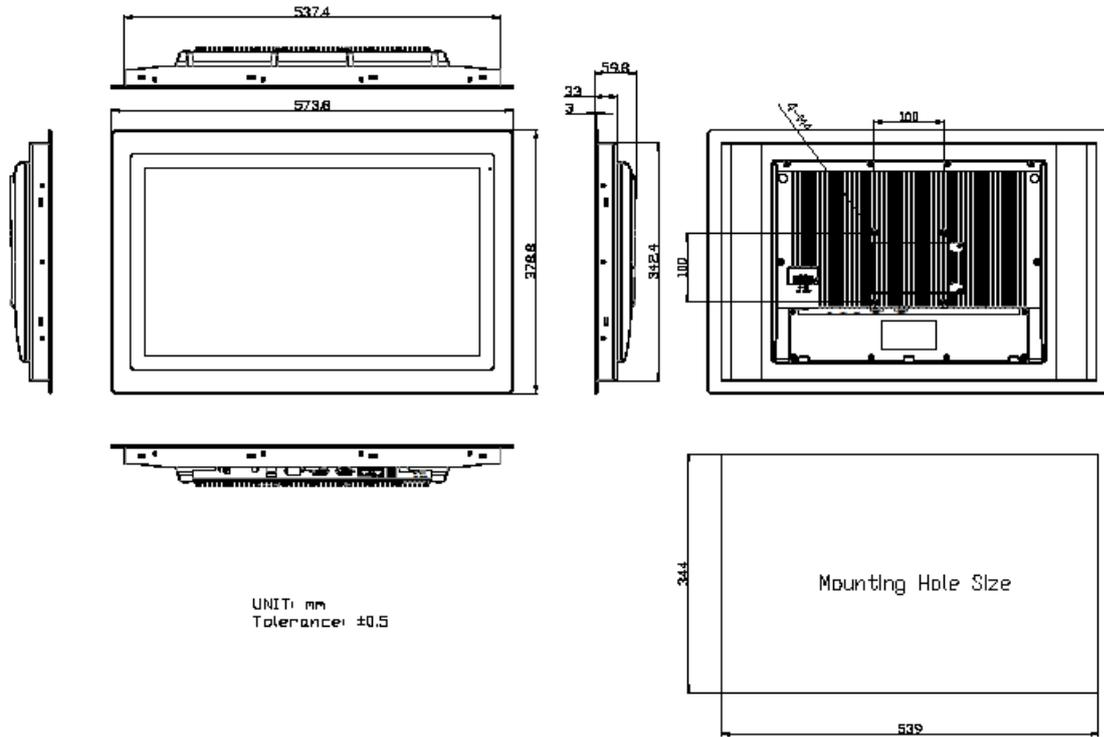
**Figure 1.7: Dimensions of FABS-821P/G(H)**
