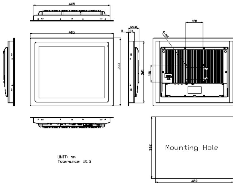
Figure 1.6: Dimensions of FABS-819P/G(H)
