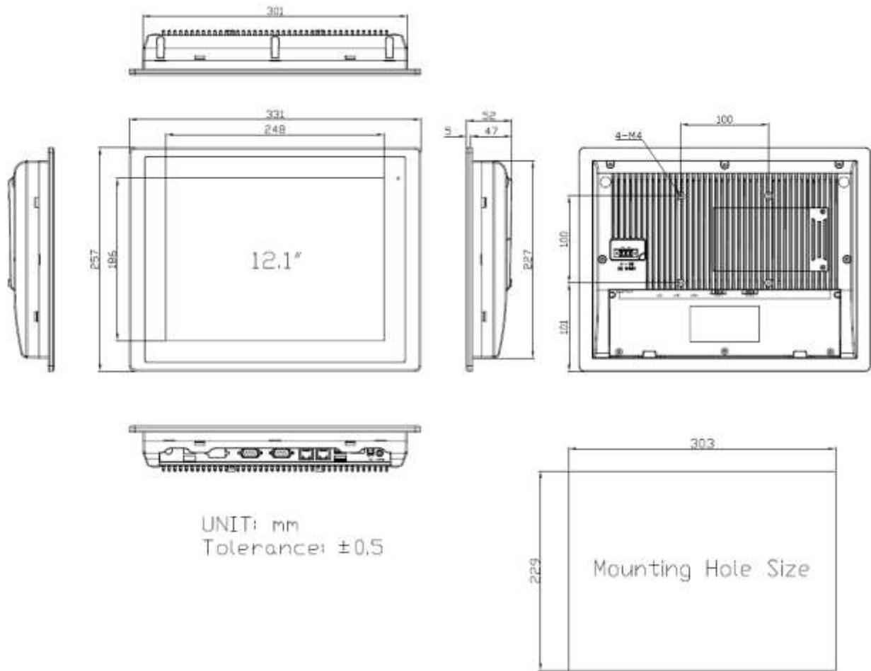
**Figure 1.3: Dimensions of FABS-812P/G(H)**
