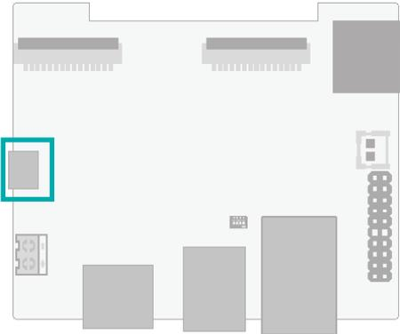
This port is for OTG programming, any USB standard Micro type interface cable or device fits the port.
