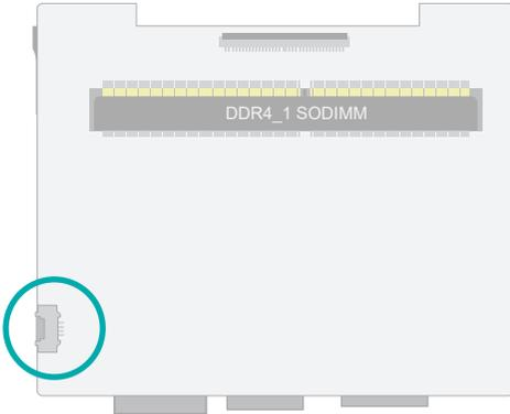
The fan connector is used to power a cooling fan. Cooling fans will provide adequate airflow throughout the chassis to prevent overheating the CPU and system board components. The 4-pin fans provide PWM to modulate fan speed.
