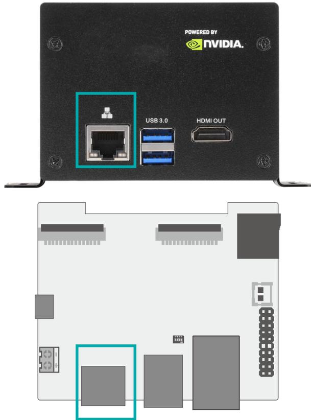
The LAN port allows the system board to connect to a local area network by means of a network hub.
