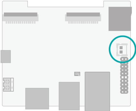
The battery supplies power to the real-time clock and CMOS memory as an auxiliary source of power when the main power is shut off.
