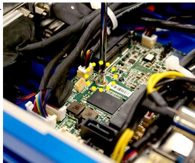
2. Insert the mSATA card into the slot at a 45-degree angle.
