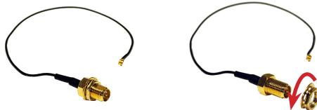
2. Assemble the antenna cables to the system front or rear panel as desired.
