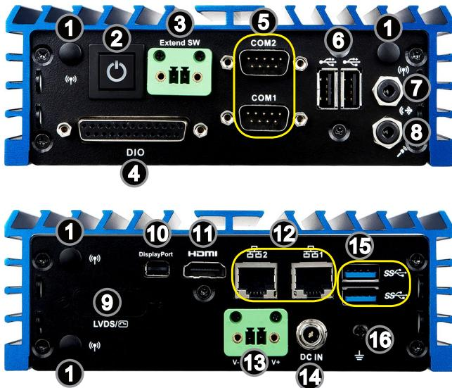
**1****WLAN Antenna Connector (Optional)**
