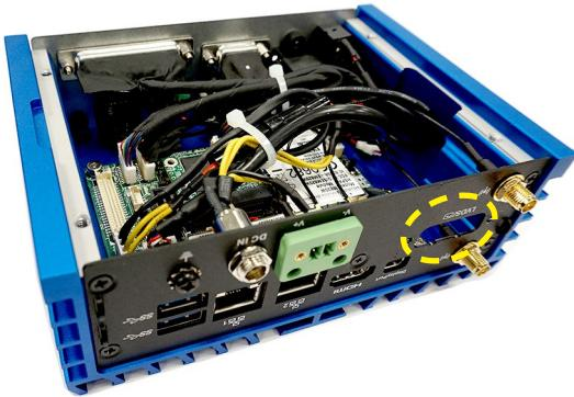
2. Secure the LVDS cable to the system rear panel with two hexagonal screws.
