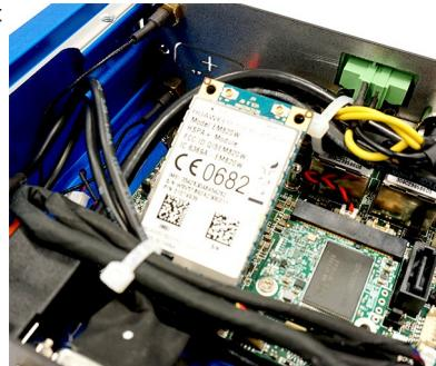
5. Push the card gently downwards and fasten it with the screw.
