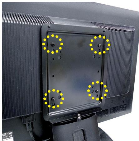
3. Install the wall mount brackets to the system.
