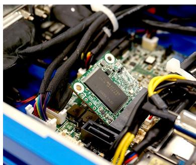
3. Push the card gently downwards and fasten it with the screw.
