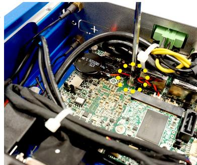
4. Insert the WiFi card into the slot at a 45-degree angle.
