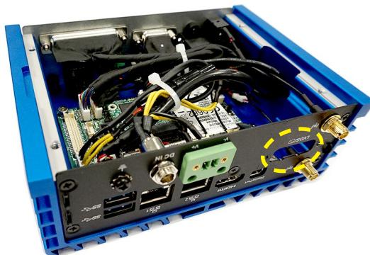
2. Secure the LVDS to DVI-I Converter Board to the system rear panel with two hexagonal screws.
