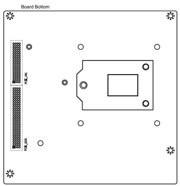
Figure 2.3: Motherboard bottom draw of ASB-M8171
