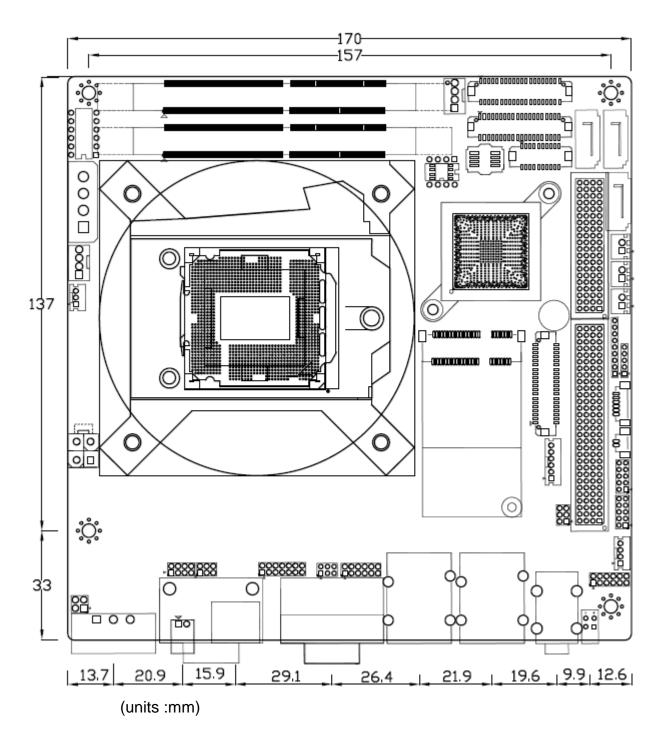
Figure 2.1: Motherboard ASB-M8171 Layout
