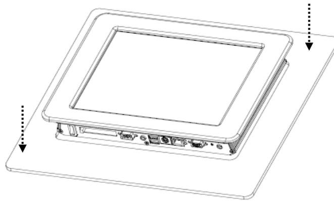
**Step 3.** Put the system into the cut-out.
