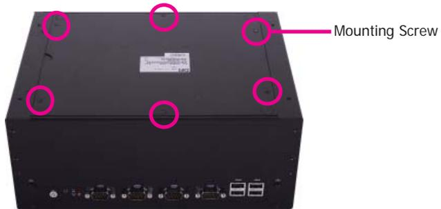
4. After removing the mounting screws, lift the cover up.
