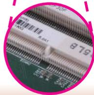
3. Grasping the module by its edges, align the module into the socket at an approximately 30 degrees angle. Apply firm even pressure to each end of the module until it slips down into the socket. The contact fingers on the edge of the module will almost completely disappear inside the socket.
