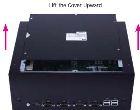
5. The SODIMM socket and the Mini PCIe slot are readily accessible after removing the chassis cover.
