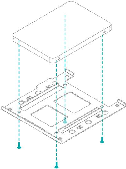
Fasten the screws and secure the drive onto the tray as illustrated with four screws.
