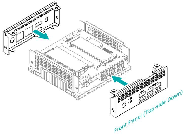
Place the assembly top-side down on a stable worksurface. Attache the front and rear panels to the assembly, and screw on the four screws as illustrated.
