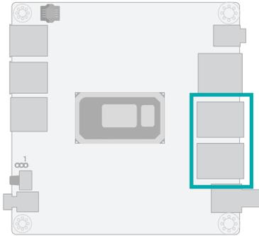
The LAN port allows the system board to connect to a local area network by means of a network hub.
