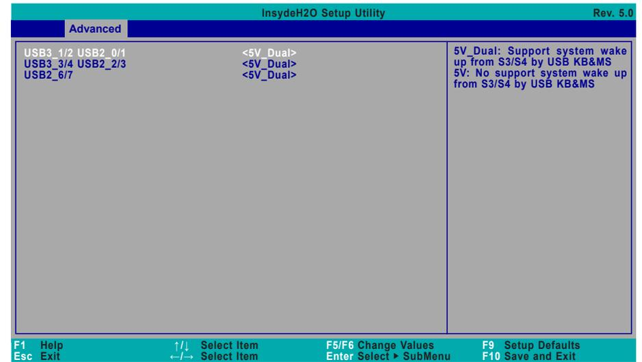
Select between 5V\_Dual and 5V for each USB controller. When Wake-on-USB from S3/S4 states is required, please select 5V\_Dual.
