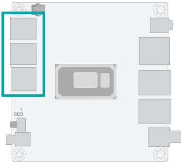
USB allows data exchange between your computer and a wide range of simultaneously accessible external Plug and Play peripherals. The system board is equipped with multiple USB Type A ports at the front panel – four USB 3.0 and two USB 2.0 ports.
