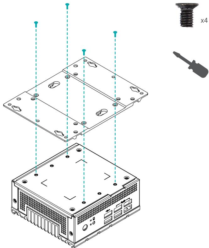
The pre-drilled mounting holes on the brackets allow for different wall mount distances. The assembly can either be screwed onto a wall or hung on steps screws.
