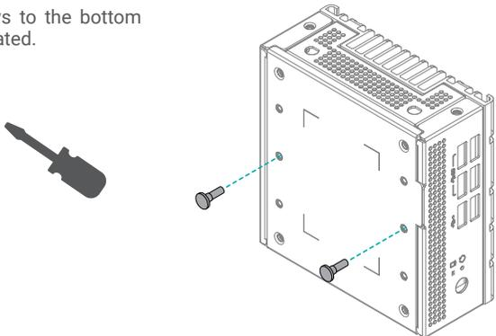
Mount the assembly onto the VESA mount bracket previously attached to the back of a monitor. Make sure the step screws sit perfectly into the step screw holes.
