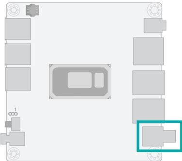
Connect the power source to the 12V DC-In coaxial. An AC-to-DC converter may be included in the package as an optional item.
