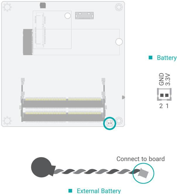
The external lithium ion battery supplies power to the real-time clock and CMOS memory as an auxiliary source of power when the main power is shut off.
