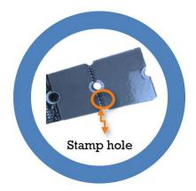
EPM-1607 is designed with 3-In-1 2280/2260/2242 & fitted in any host computer that has M.2 slots. If user's device has M.2 2242 or 2260 socket, you can easily to break-away EPM-1607 PCB with Stamp hole design & modify M.2 card from size 2280 to 2260 or 2242.
