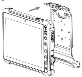
2 Make sure the tablet is firmly inserted into the cradle.
