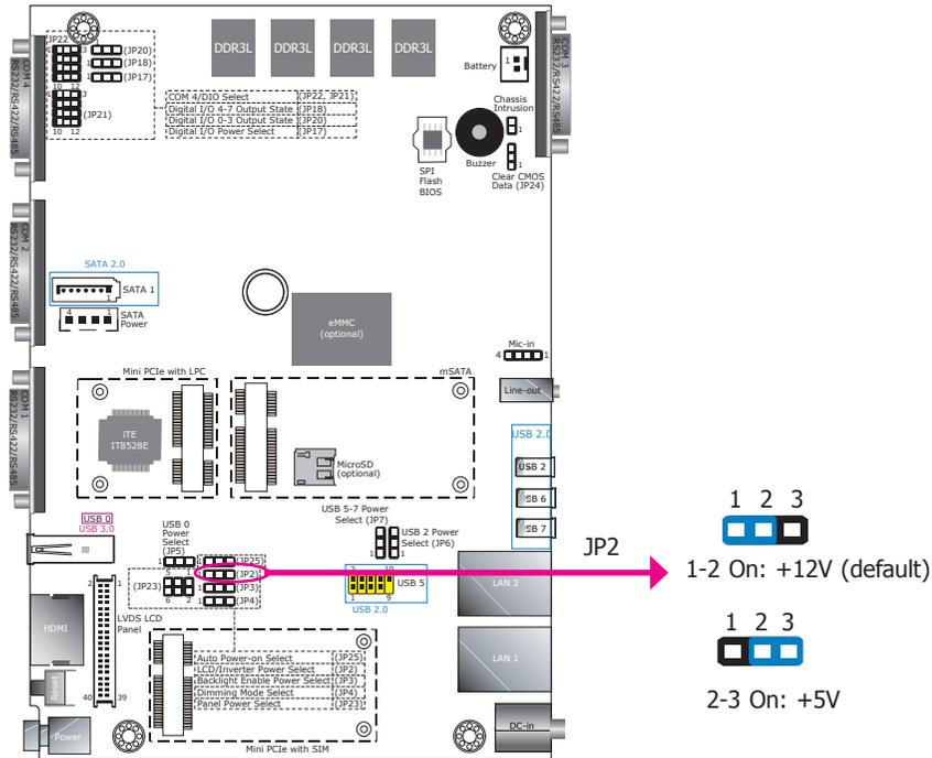
JP2 is used to select the power level of the LCD/inverter power connector.
