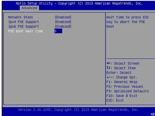
When the Network Stack is set to enabled, it will display the following information:
