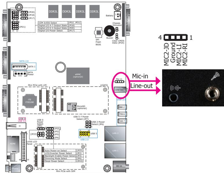
This Line-out jack is used to connect a headphone or external speakers. And the MIC-in connector is used to connect an external microphone. The audio ports are built based on the Realtek ALC888 chipset.
