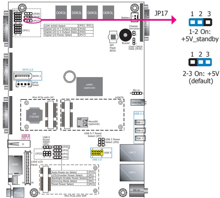
JP17 is used to select the power of the DIO (Digital Input/Output) signal.
