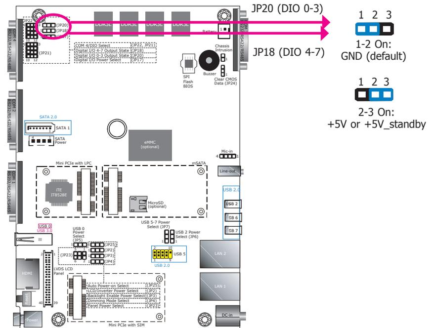
Based on the power level of DIO (Digital I/O) selected on JP17, JP20 (for DIO pin 0-3) and JP18 (for DIO pin 4-7) are used to select the state of DIO output: pull-high or pull-low. When selecting pull-high, the power selection will be set according to JP17's setting.
