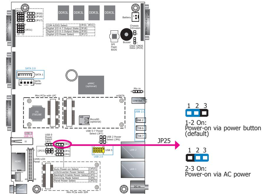
JP25 is used to select the method of powering on the system. If you want the system to power on whenever AC power comes in, set JP25 pins 2 and 3 to On. If you want to use the power button, set pins 1 and 2 to On.
