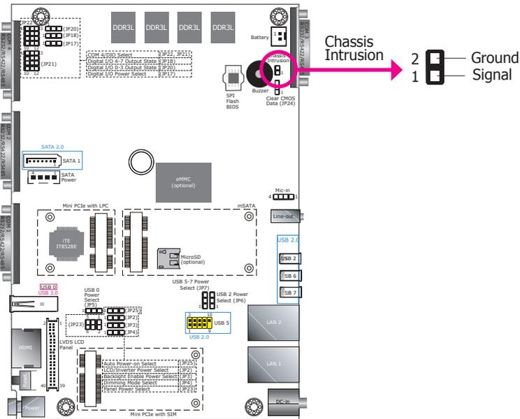
The board supports the chassis intrusion detection function. Connect the chassis intrusion sensor cable from the chassis to this connector. When the system's power is on and a chassis intrusion event occurs, an alarm will sound. When the system's power is off and a chassis intrusion event occurs, the alarm will sound only when the system restarts.
