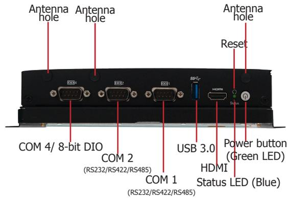
The top panel I/O consists of the following ports and connectors:
