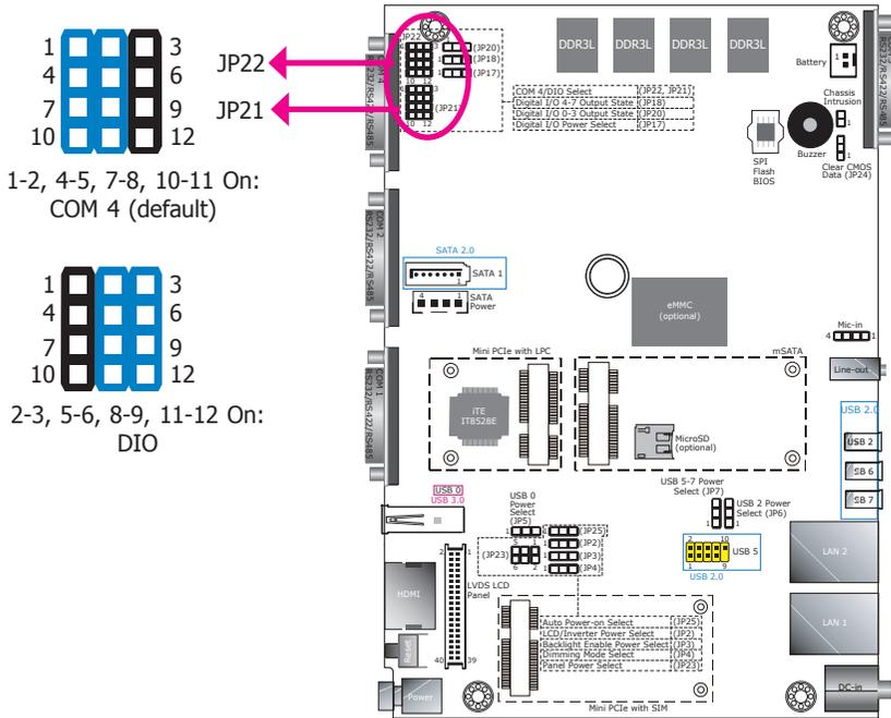
The system board uses JP21 and JP22 to select between RS232/422/485 COM 4 or an 8-bit DIO connector.
