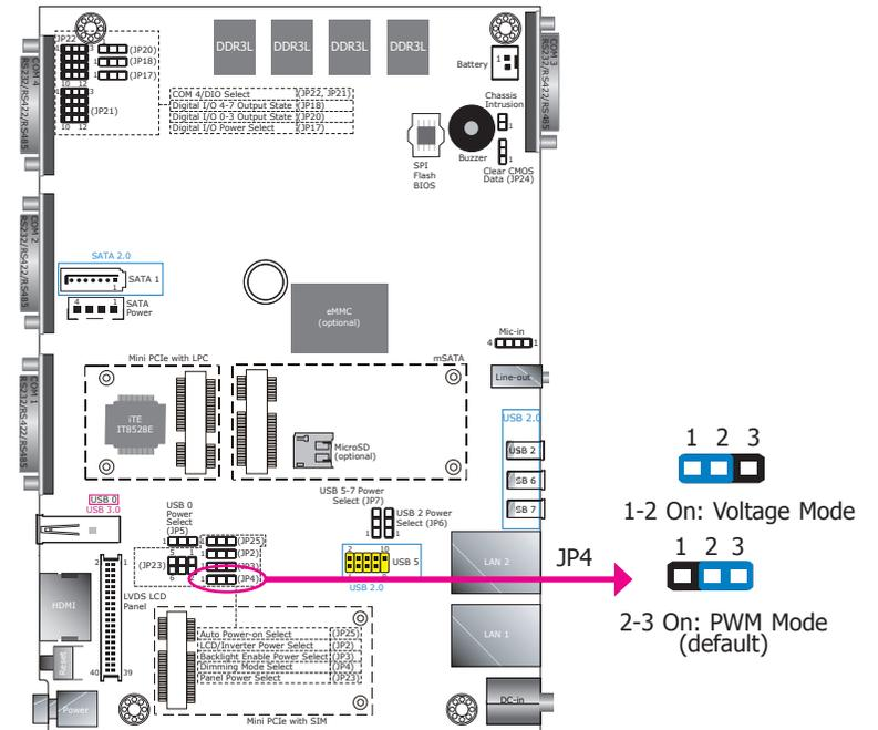
JP4 allows you to select the mode for the backlight brightness control of the LVDS panel.
