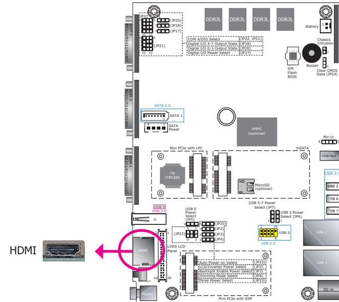
The HDMI port, which carries both digital audio and video signals, is used to connect a LCD monitor or digital TV.
