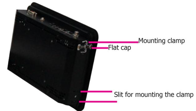
5. Position the mounting clamps along the rear edges of the Panel PC and insert them into the slits around the Panel PC.
