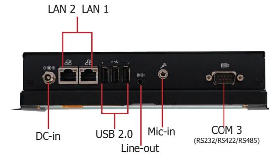
The bottom panel I/O consists of the following ports and connectors:
