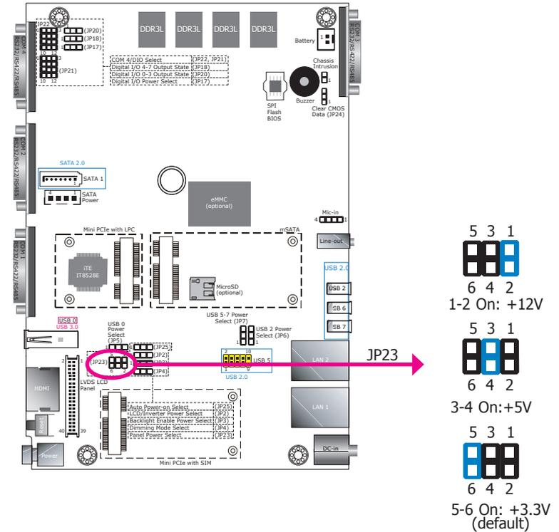
JP23 is used to select the power supplied with the LCD panel.
