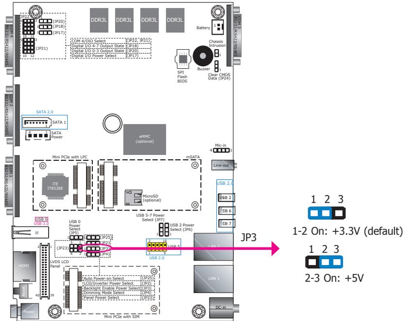
JP3 is used to select the power level of backlight brightness control: +5V or +3.3V.
