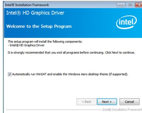
By default, the "Automatically run WinSAT and enable the Windows Aero desktop theme" is enabled. When this is enabled and the system reboots after driver installation, the screen will turn blank for 1 to 2 minutes (while WinSAT is running) before the Windows 7/ Windows 8 desktop appears. The "blank screen" period is the time Windows is testing the graphics performance.
