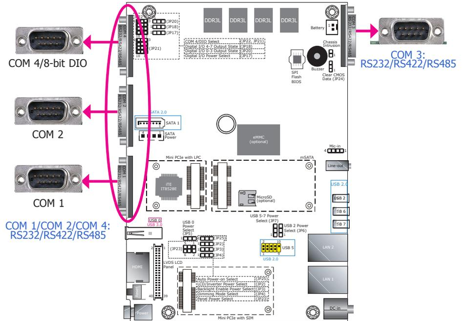
The serial ports are asynchronous communication ports with 16C550A-compatible UARTs that can be used with modems, serial printers, remote display terminals, and other serial devices.
