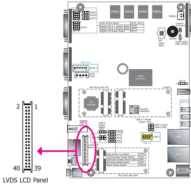
The system uses this connector as the output interface of the touch panel PC. It transmits video signals and power from the system board to the display panel.
