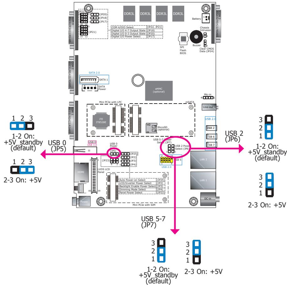
JP5, JP6 and JP7 are used to select the power for the USB ports of USB 0, USB 2 and USB 5-7 respectively. Selecting +5V\_standby will allow you to use USB devices to wake up the system.
