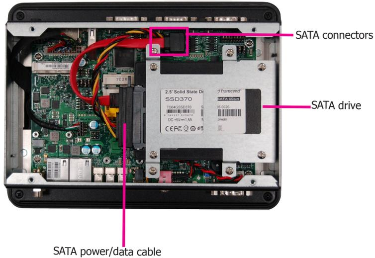
4. Align the mounting holes of the HDD drive bay with the mounting holes on the system and use the provided mounting screws to secure the drive bay in place.
