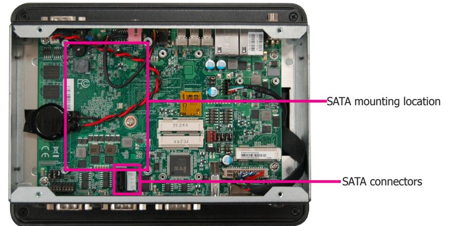
2. Align the mounting holes of the SATA HDD with the mounting holes on the HDD drive bay and use the provided mounting screws to attach the SATA HDD to the drive bay.
