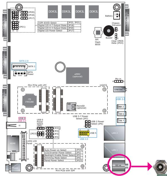
Connect a DC power cord to this jack. Use a power adapter within 16~24V DC output voltage. Using a power adapter that does not conform to the specified voltage may fail to boot the system or cause damage to the system board.
