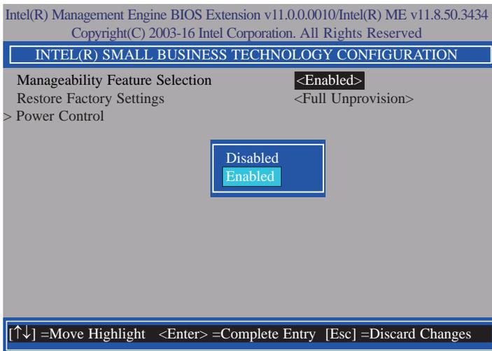
15. In the **Intel(R) Small Business Technology Configuration** menu, select **Power Control** then press Enter. In the **Intel(R) AMT Power Control** menu, select **Intel(R) AMT ON in Host Sleep States** then press Enter. Select an option then press Enter.
