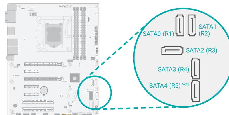
The Serial ATA (SATA) connectors are used to connect the Serial ATA device. SATA 3.0 is supported by the five SATA ports and provides data rate up to 6Gb/s. Connect one end of the Serial ATA cable to a SATA connector and the other end to your Serial ATA device.
