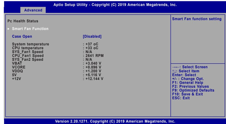
This section displays the system's health information, i.e. voltage readings, CPU and system temperatures, and fan speed readings.
