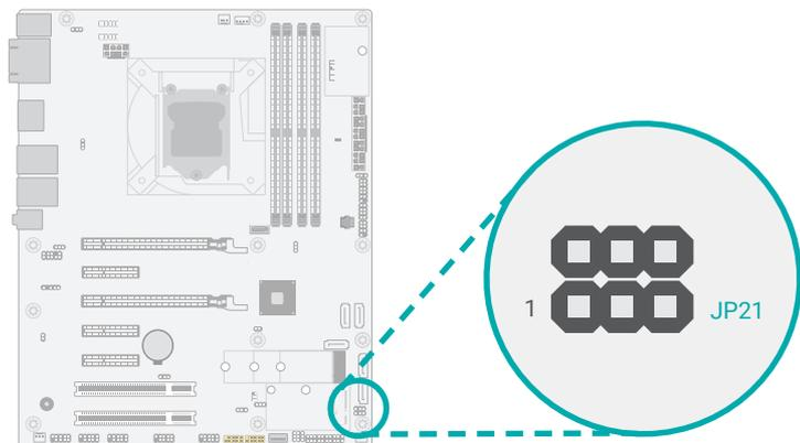
The signal of Mini PCIe can be switched between mSATA (default) or PCIe via JP21.
