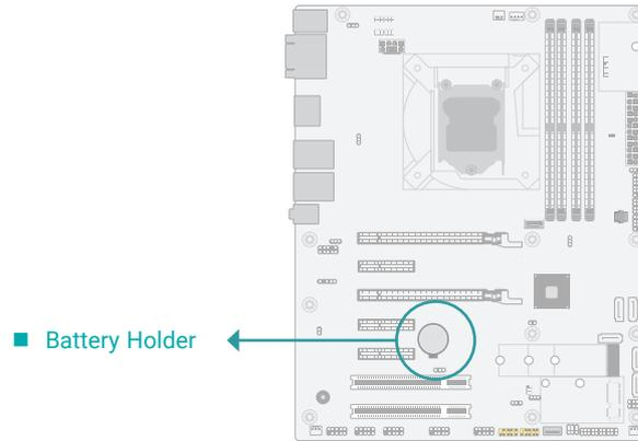
The lithium ion battery addendum supplies power to the real-time clock and CMOS memory as an auxiliary source of power when the main power is shut off. Insert a coin cell battery into the holder and make sure the polarities are correctly oriented – the cap side (rimmed rounded edge) is negative and should be facing the holder; the flat side with a + mark is positive and should be facing away from the holder.
