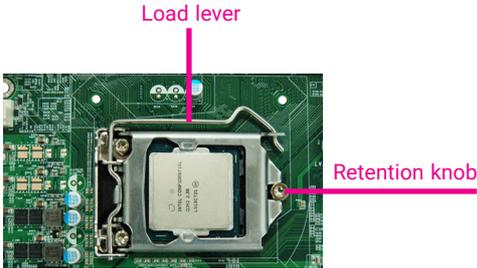
9. Press down the load lever and hook it under the retention tab.
