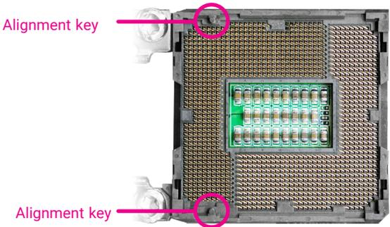
7-3. The CPU's notch will fit into the socket's alignment key when it's seated in the correct orientation.
