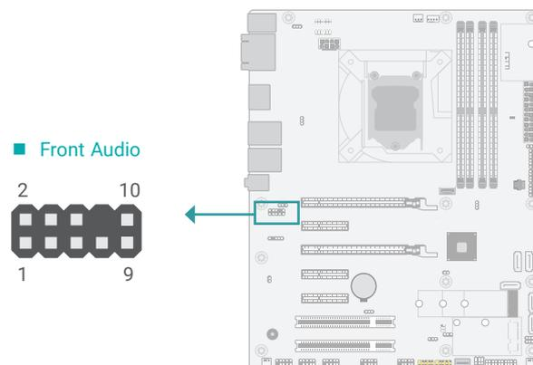
The Front Audio internal connector allows you to connect to the second line-out and mic-in jacks that are at the front panel of your system.
