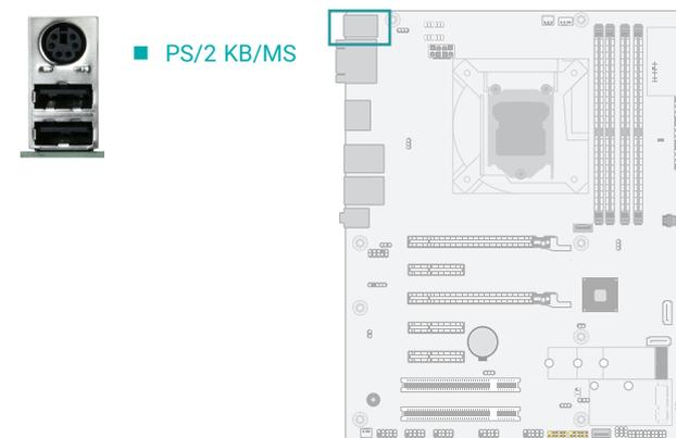
This rear I/O port is used to connect a PS/2 keyboard/mouse. IRQ12 is reserved for the PS/2 mouse connector.
