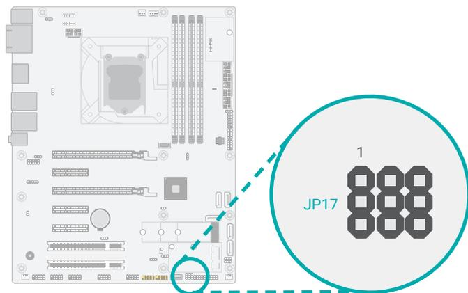
JP17 is used to select the power of Digital I/O: +5V<sub>DU</sub> (default) or +5V.
