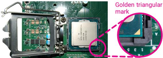
**Important:** The CPU will fit in only one orientation and can easily be seated without exerting any force.
