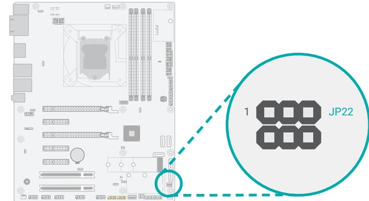
The power of Mini PCIe can be switched between 3V3DU and 3V3 via JP22.
