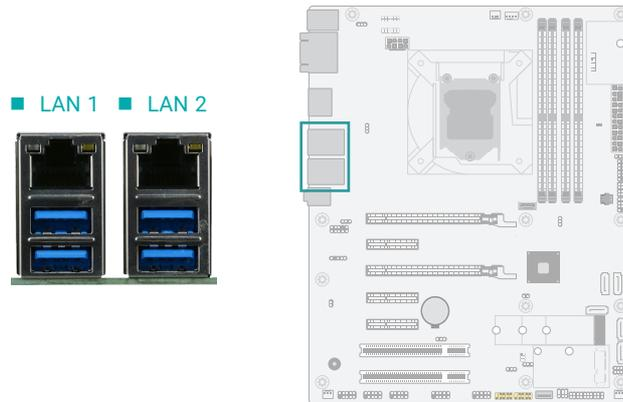
The two LAN ports allow the system board to connect to a local area network.
