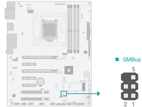
The SMBus (System Management Bus) connector is used to connect the SMBus device. It is a multiple device bus that allows multiple chips to connect to the same bus and enable each one to act as a master by initiating data transfer.
