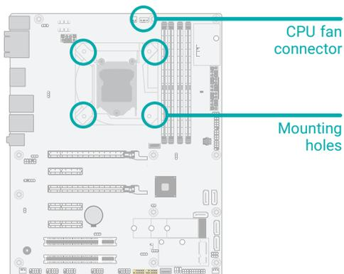
4. Screw tight two of the spring screws at opposite corners into the mounting holes. And then proceed with the other two spring screws.
