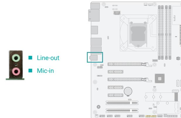
The system board is equipped with three rear audio jacks:
