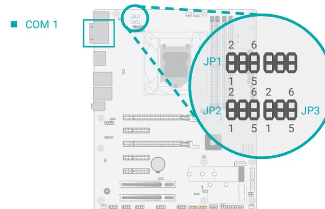
JP1, JP2, and JP3 are used to configure the COM 1 port to RS232 (Full Duplex) or RS485. The three jumpers must all be configured to the same serial mode.
