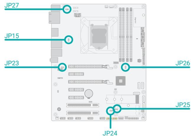
The power of the USB connectors' voltage buses can be configured to either 5V<sub>DU</sub> or 5V. The jumpers are located as illustrated above and correspond to each USB port number as listed.
