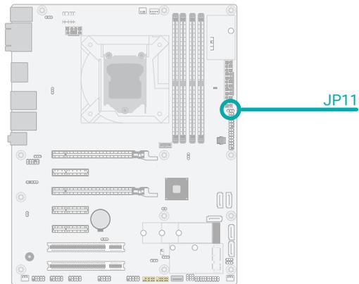
Power of the system can be turned on via the Power Button or via the AC-In signal. Switch the setting by putting the jumper caps on neighboring pins of JP11 as listed and illustrated below:
