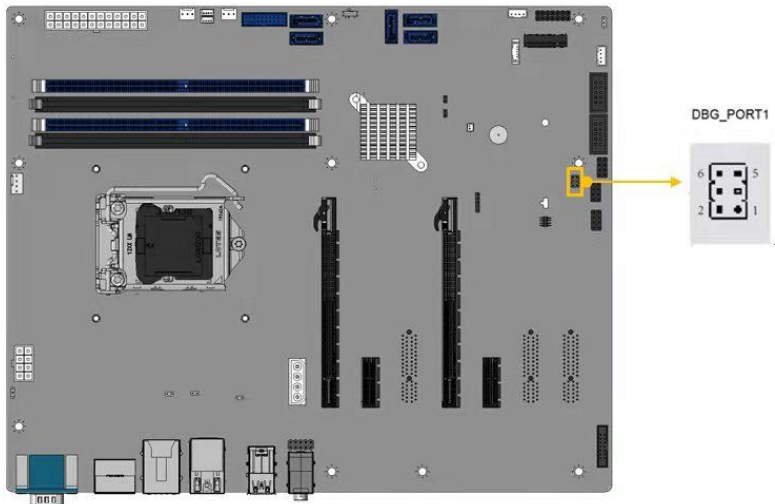
Figure 3-9: Debug Connector Location
