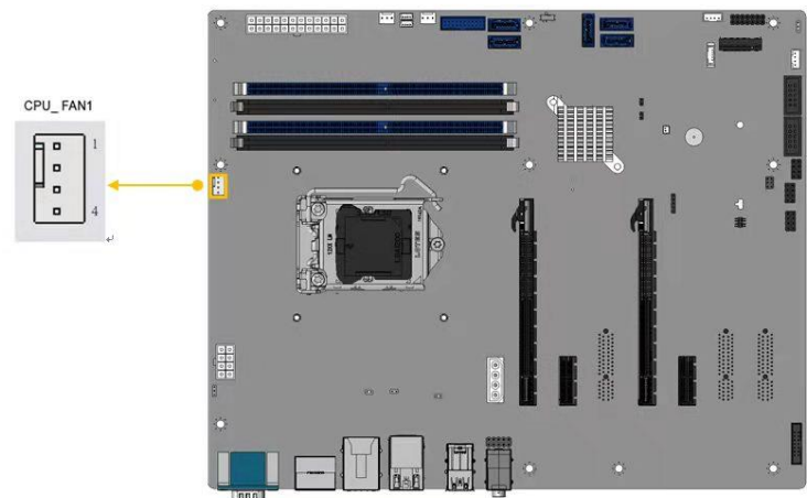
Figure 3-11: CPU Fan Connector Location
