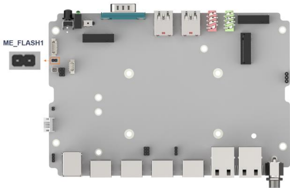
Figure 3-21: Flash Descriptor Override Setting Jumper Location
