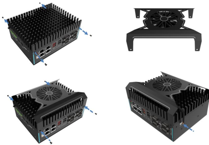
Figure 3-9: External Fan Module Installation
