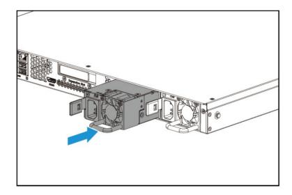
Step 4: Connect the power adaptor and cables to the GRAND-GL.
