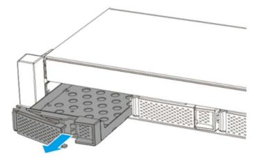
**Step 3:** Install a 3.5" or 2.5" disk drive on the drive tray.
