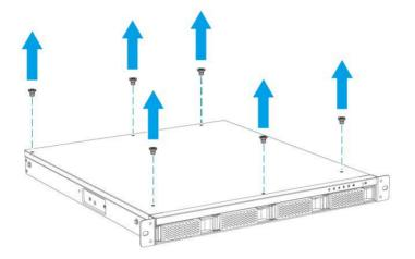
Figure 3-1: Case Cover Retention Screws
