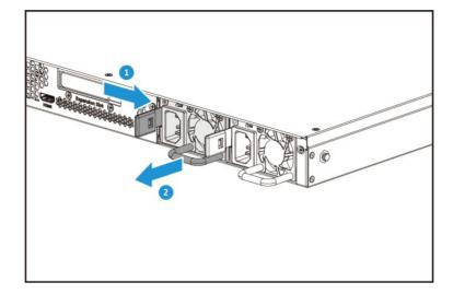
Step 3: Insert new power supply into the GRAND-GL.
