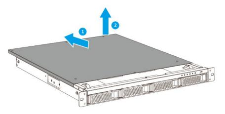
Figure 3-2: Remove the Case Cover
