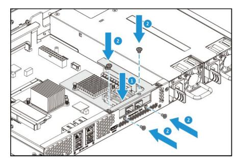
Step 6: Insert the riser card into the slot. Attach the screws.
