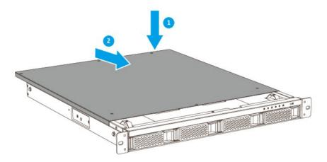
Figure 3-3: Place and Slide the Cover
