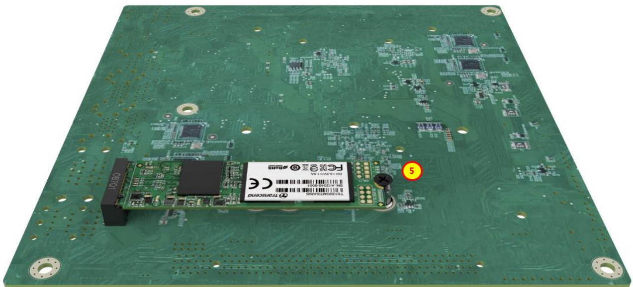
Figure 4-9: Securing the M.2 Module
