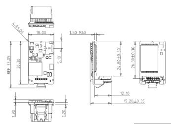
TOLERANCE: ±0.20mm UNIT: mm
