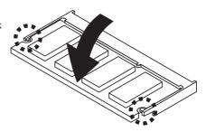
3. To uninstall the DIMM, flip the slot levers outwards and the DIMM will be released instantly.
