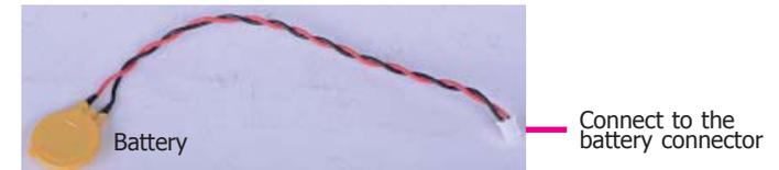
The lithium ion battery powers the real-time clock and CMOS memory. It is an auxiliary source of power when the main power is shut off.
