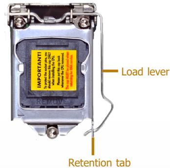
5. Lift the load lever and the load plate all the way up as shown in the photo.
