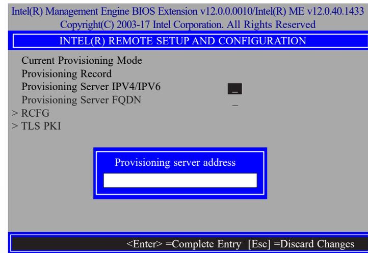
42. In the **Intel(R) Remote Setup And Configuration** menu, select **Provisioning Server FQDN** then press Enter. Enter the FQDN then press Enter.
