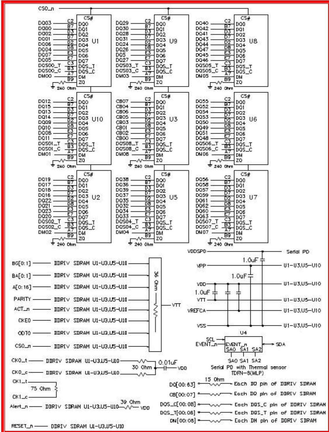
Note: 1. The ZQ ball on each DDR4 component is connected to an external 240Ω ±1% resistor that is tied to ground. It is used for the calibration of the component's ODT and output driver.
