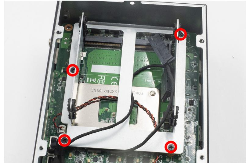
6. To install or replace the SO\_DIMM2, remove the 4 screw around the 2.5" slots first, and tilt up the slot.
