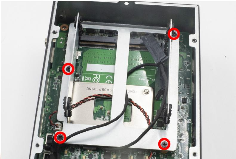
8. Then you can install the memory on the SO\_DIMM2 slot.
