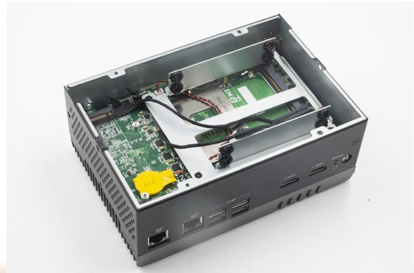
5. There are two M.2 slots and an InnoAGE HDR1 pinout on the board.
