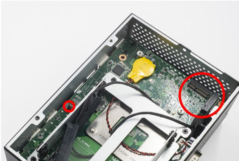
7. To install or replace the SO\_DIMM2, remove the 4 screw around the 2.5" slots first, and tilt up the slot.
