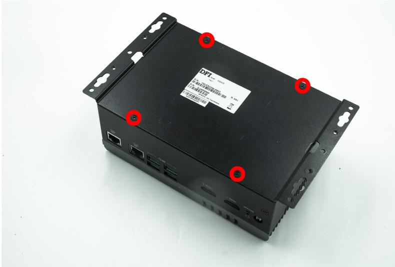
2. If you need to install or replace the CPU and 2nd memory, please also remove the three screws at each side of the box.
