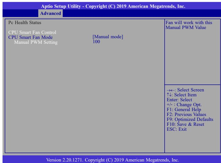
When "CPU Smart Fan Mode" is set to "Manual mode", the following field will appear.
