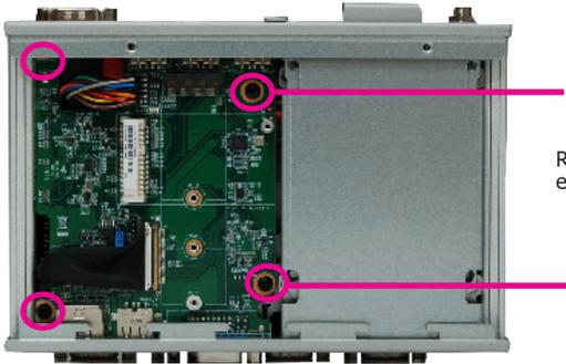
Remove these screws to detach the expansion board from the main board
