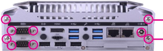
Use a wrench to remove the hexagonal gasket
