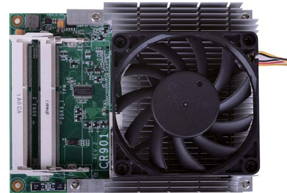
Top View of the Heat Sink
