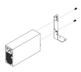
**Step 2: Install the power supply to the chassis.** Secure the power supply to the chassis with the screws as figure shown below.
