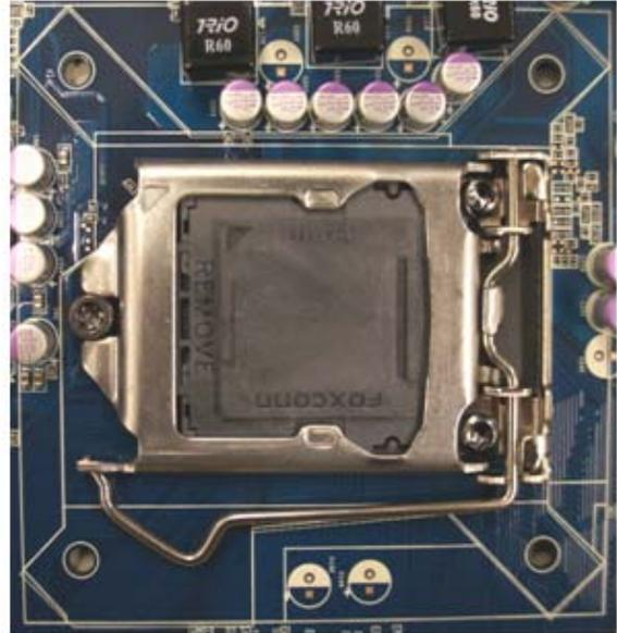
2. Unlatch the "CPU Socket Lever" by pressing the lever down and move it away from the main structure of the socket.
