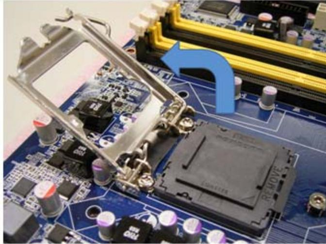
4. The CPU socket has a plastic protection cap installed on it (black color, a.k.a. “CPU Socket Cover”, or “PnP cap”) in order to protect the socket pins from damage. If you are going to install a CPU, remove the plastic protection cap away from the CPU socket by lifting it up
