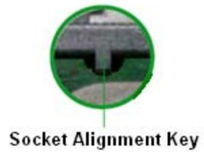
6. Visually inspect if the CPU is seated into the CPU socket evenly. The “Socket Alignment keys” should fit into the CPU notches.
