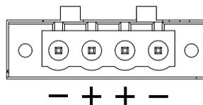
Figure 2.7 4-Pin Header
