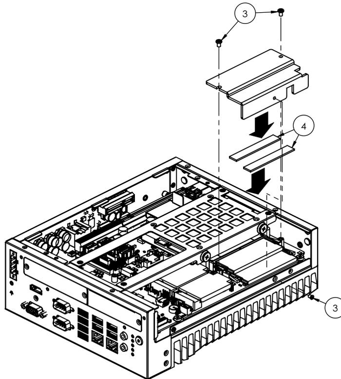
3. Undo 3 screws to remove the memory thermal cover.
