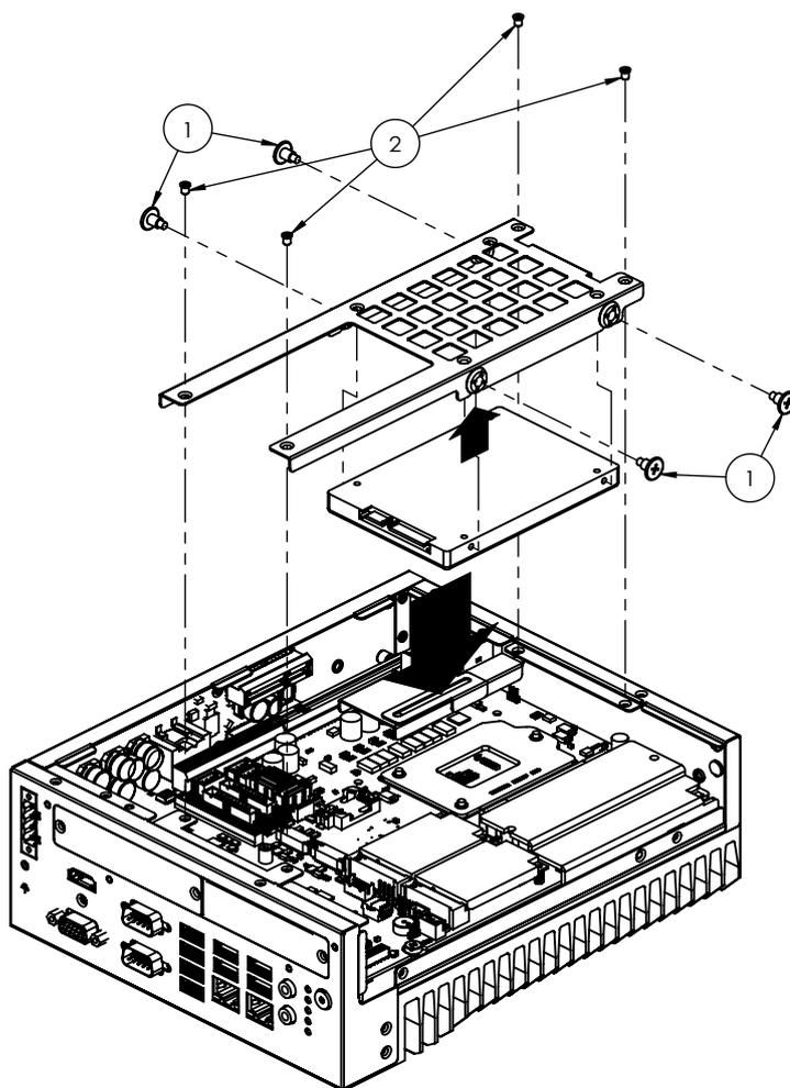
3. Secure the HDD with 4 x HDD screws (P/N:1930002235).
