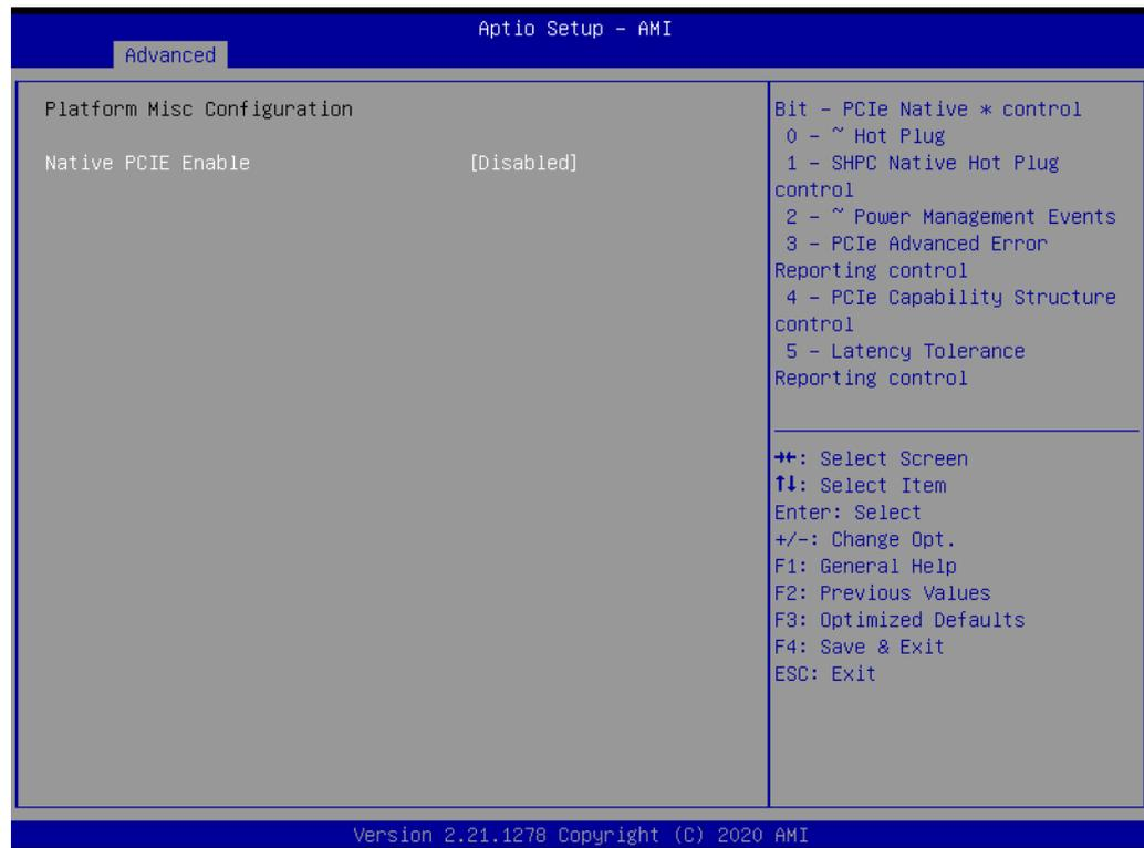
Figure 3.5 Platform Misc Configuration
