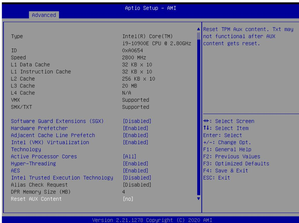
**Figure 3.6 CPU Configuration**
