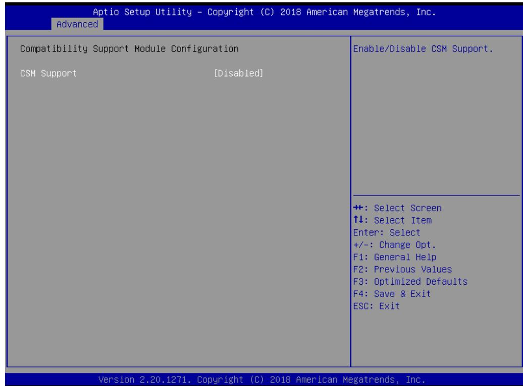
**Figure 3.34 CSM Configuration**
