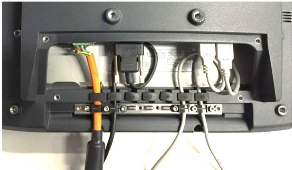
Fig. 15.9: Cables and dummy grommets
