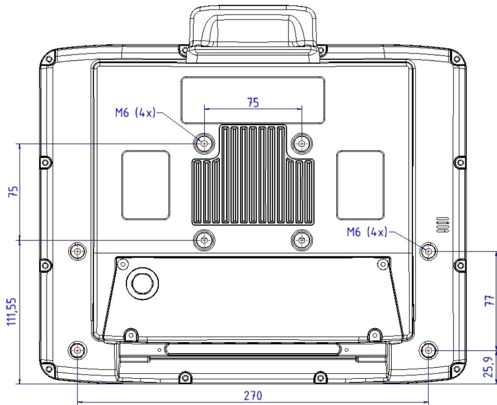
Fig. 13.2: Position of the VESA drill holes DLT-V8312
