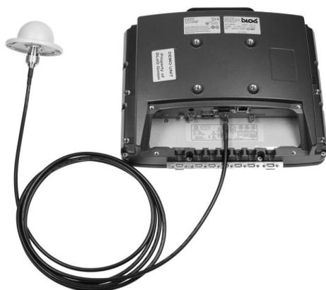
Fig. 6.5: External WLAN antenna (optional)
