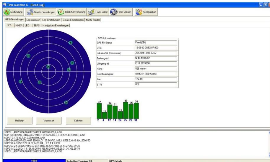
Fig. 6.9: Ext. GPS receiver, display example during installation
