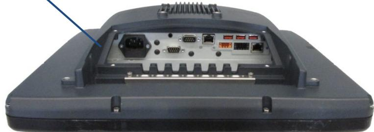
Fig. 5.8: AC power connector with detail view
