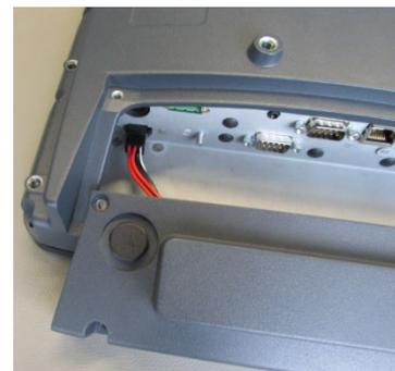
Fig. 15.11: Cable cover with integrated UPS battery
