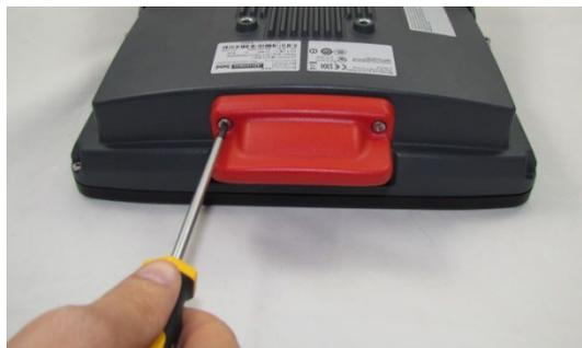
Fig. 8.2: Open WLAN antenna IEEE 802.11 a/b/g/n/ac
