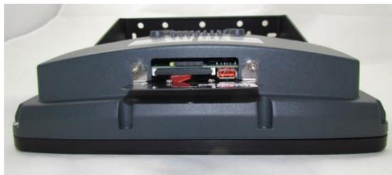
Fig. 8.3: WLAN antenna IEEE 802.11 a/b/g/n/ac opened
