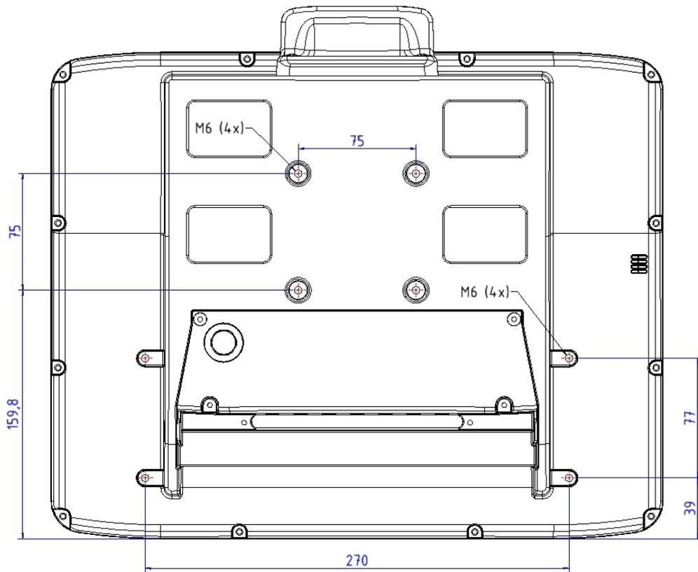
Fig. 13.3: Position of the VESA drill holes DLT-V8315
