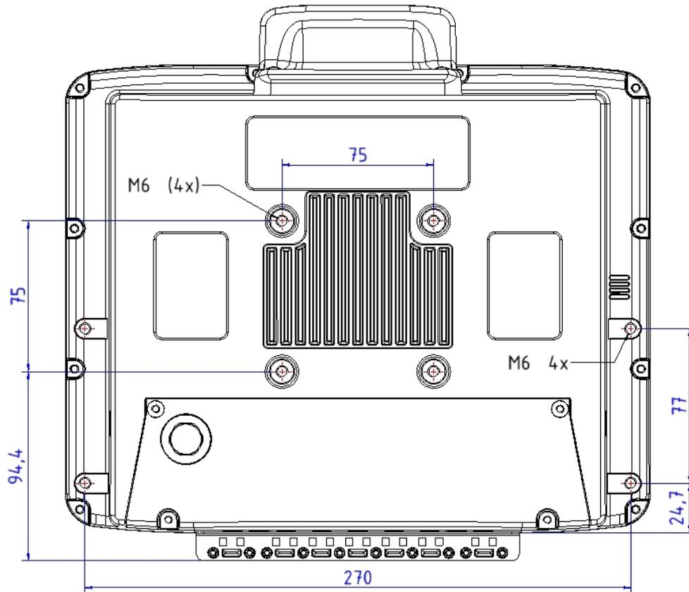
Fig. 13.1: Position of the VESA drill holes DLT-V8310
