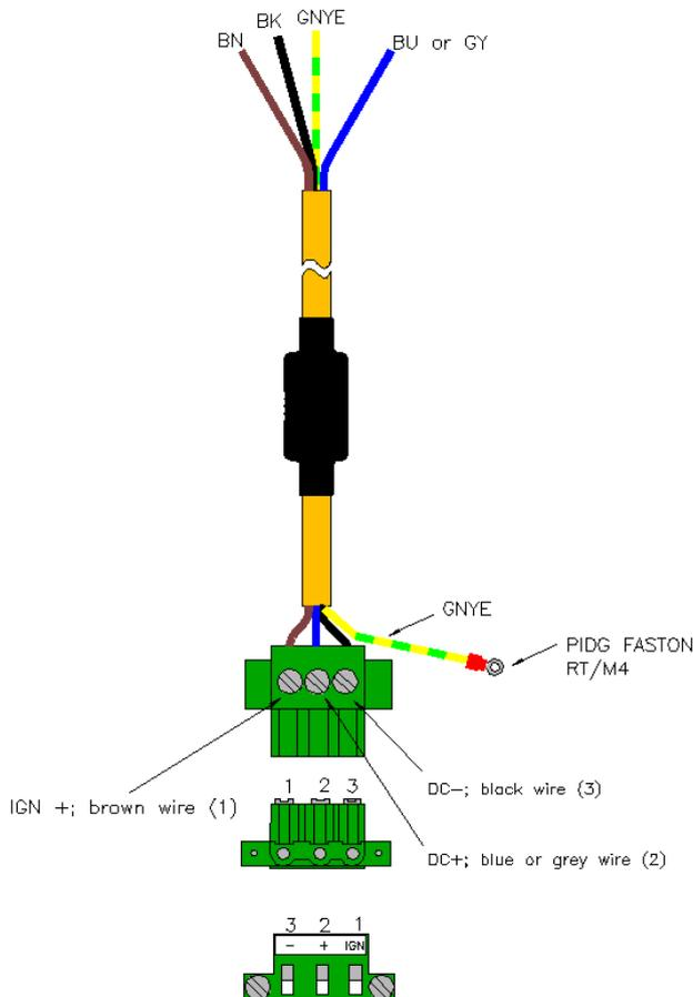
Fig. 5.7: DC connection cable assignment - drawing
