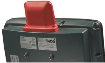
Fig. 8.4: WLAN, WWAN 3G antenna
