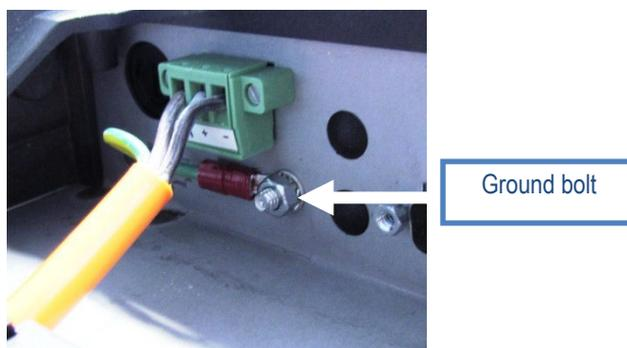
Fig. 14.2: Position of the ground bolt
