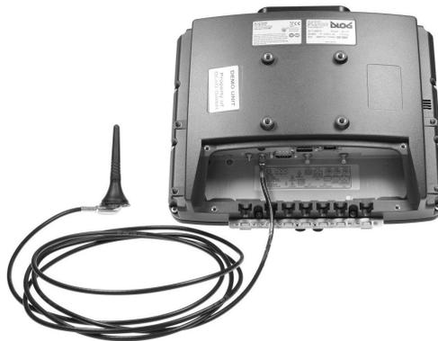
Fig. 6.6: External 3G WWAN antenna (optional)
