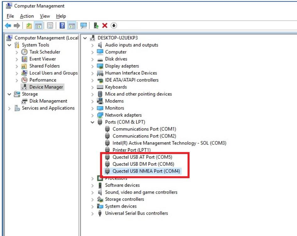
Fig. 12.21: QUECTEL EC25 - Virtual COM ports DLT-V83 with i5 processor
