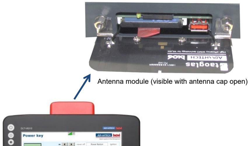
Fig. 6.2: WLAN antenna IEEE 802.11 a/b/g/n/ac and antenna module (optional)
