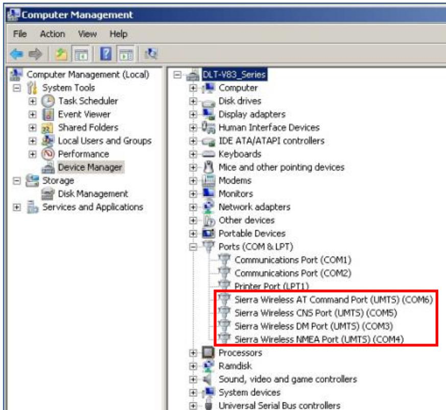
Fig. 12.10: SIERRA WIRELESS MC80 - Virtual COM ports DLT-V83 with D525 processor
