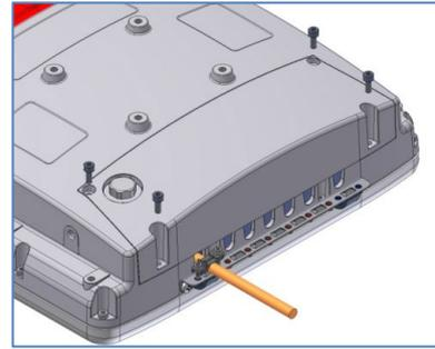
Fig. 15.10: Screwing the cable cover into place
