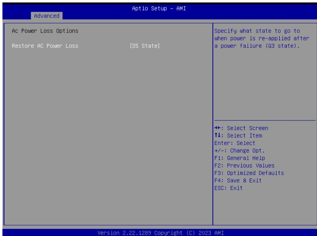
**Figure 3.11 Ac Power Loss Options**
