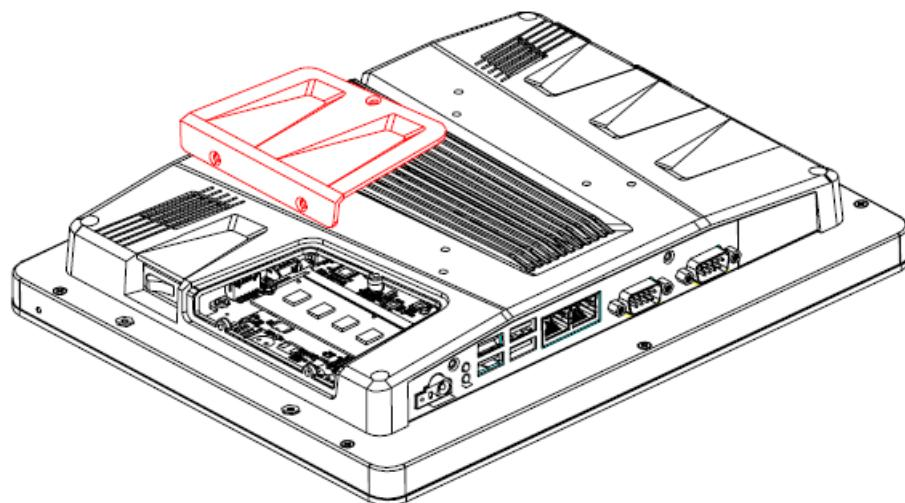
**Step 2.1** Insert the SODIMM into the memory socket.
