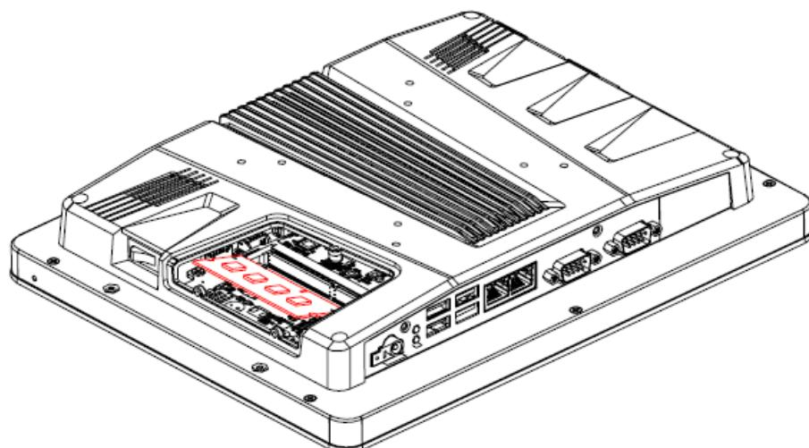
**Step 3. HDD Installation:** Insert the HDD into the Drive Bay and fasten 2 screws.
