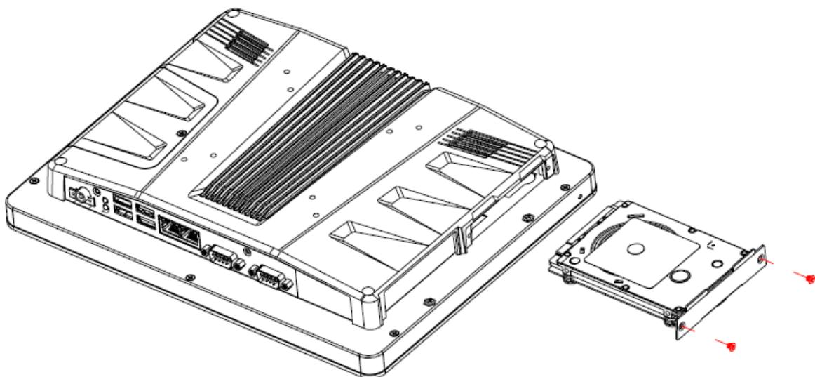
**Step 2.** Remove 4 screws to release the chassis cover, and remove it.
