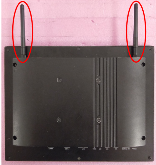
Figure 2.17 Assemble WiFi Antenna
