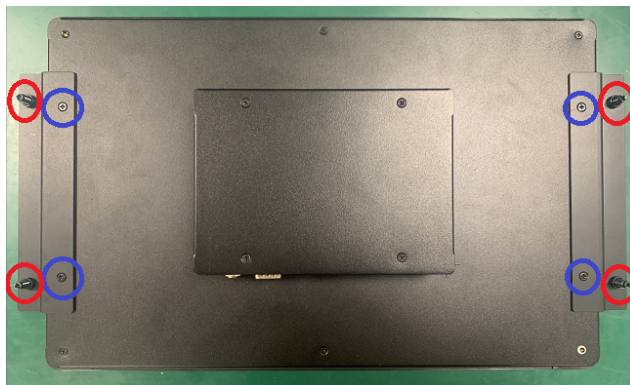
Figure 2.20 Install panel mount bracket
