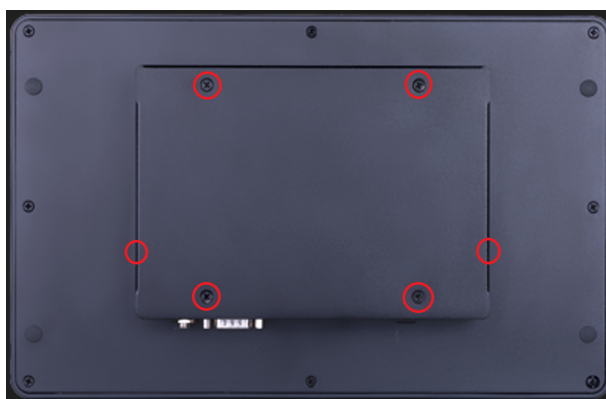
Figure 2.3 Retention screws on rear cover
