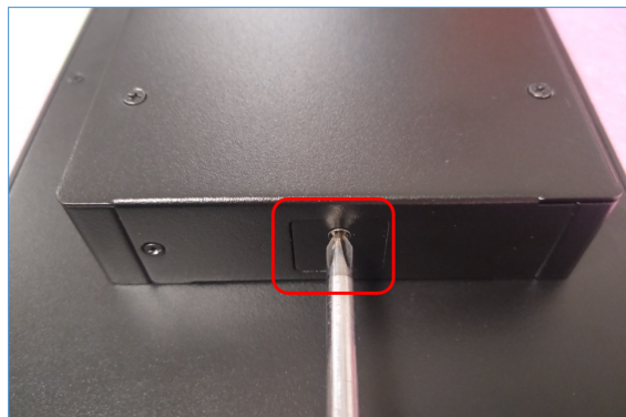
Figure 2.1 Remove SD card bracket
