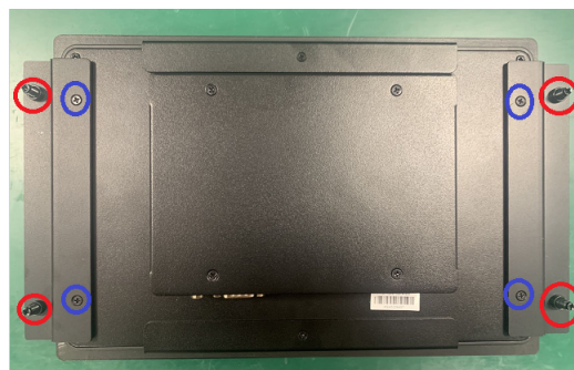
Figure 2.14 Install panel mount bracket
