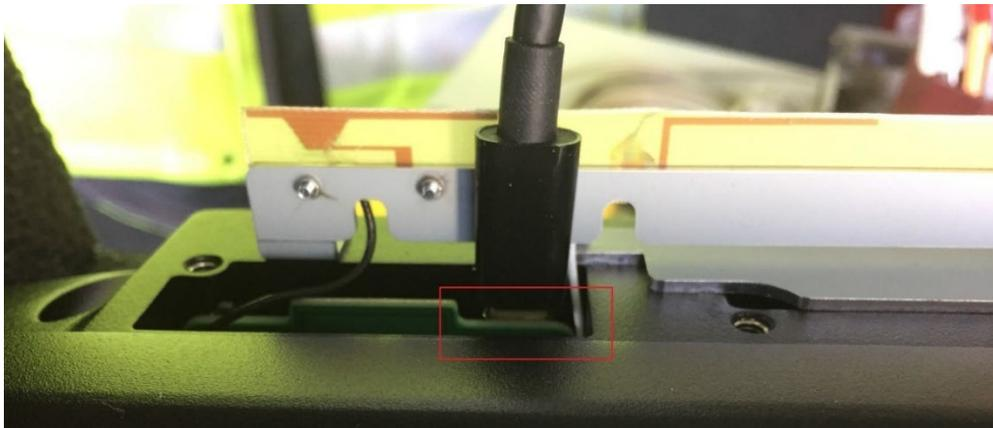
Figure 7-33: USB cable connected to port (top view)
