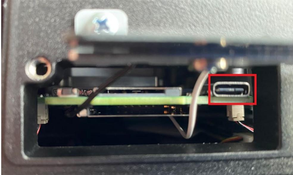
Figure 7-32: USB-C connector (top view)
