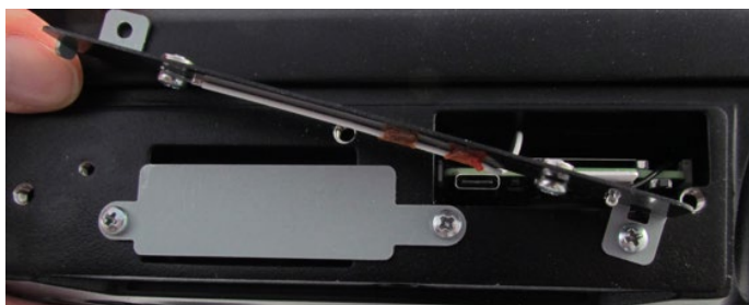
Fig. 15-4: Opened WLAN Diversity Antenna
