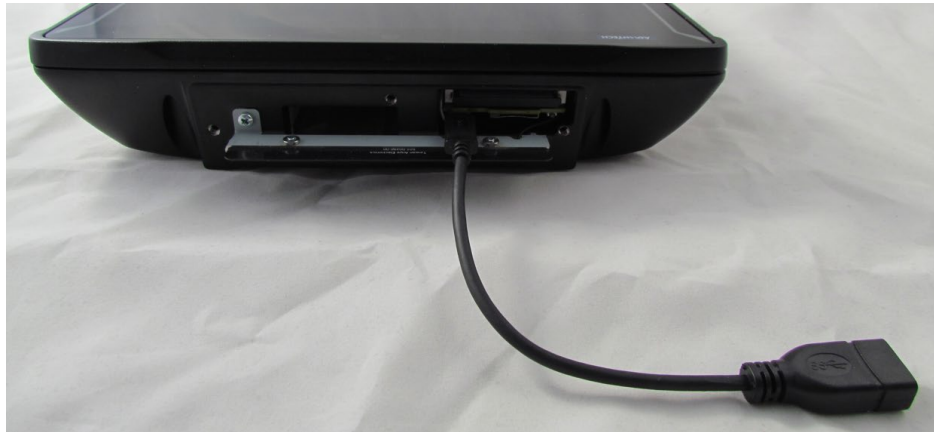
Fig. 7-23: Connected adapter to USB Type-C Service Port
