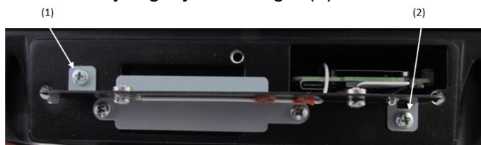
Fig. 15-3: WLAN Diversity Antenna
