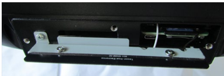
Fig. 7-22: WLAN antenna cap IEEE 802.11 a/b/g/n/ac opened
