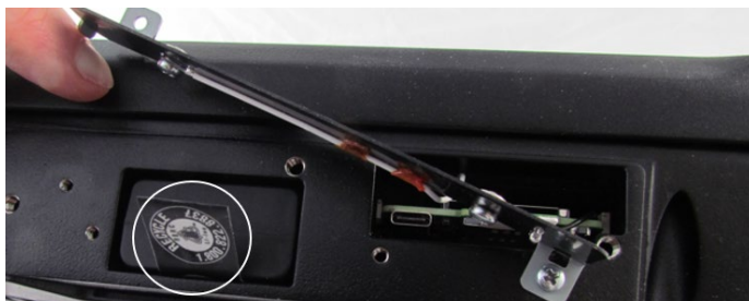
Fig. 15-7: Inserted battery pack
