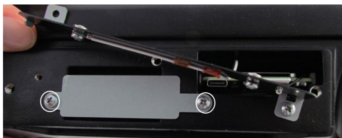
Fig. 15-5: Screws from the battery cover
