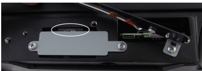
Fig. 15-8: Removal tab under the battery cover
