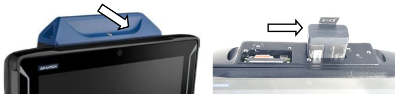
Fig. 15-1: Battery pocket with UPS DLT-V73A
