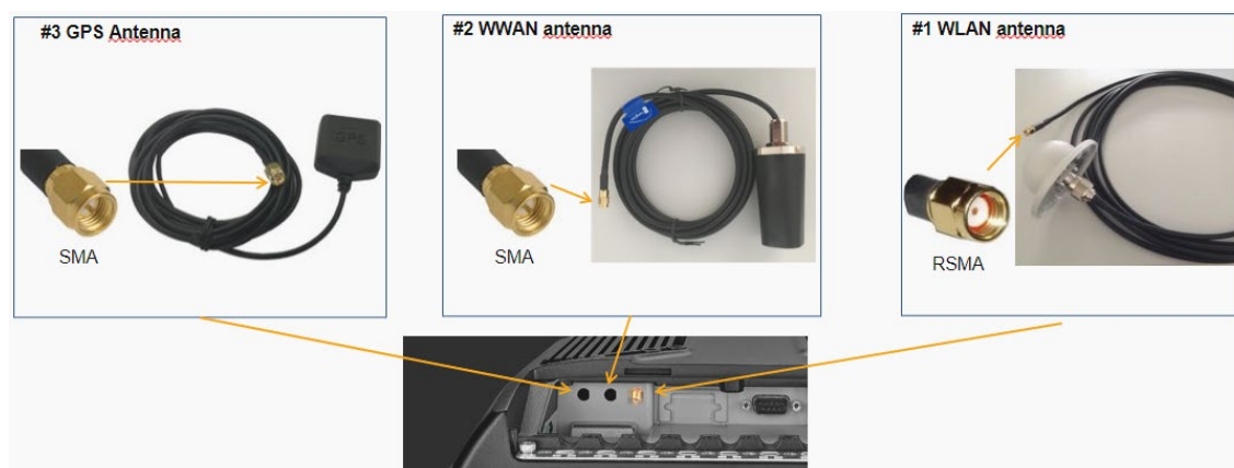
Fig. 7-4: Pin assignment description external antennas
