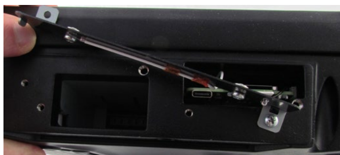
Fig. 15-6: Opened battery compartment
