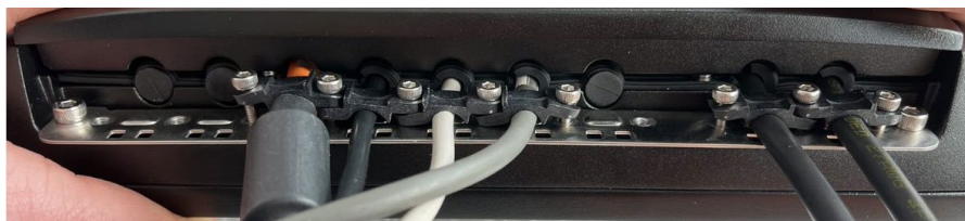
Fig. 14-14: Cable cover closed and screwed together
