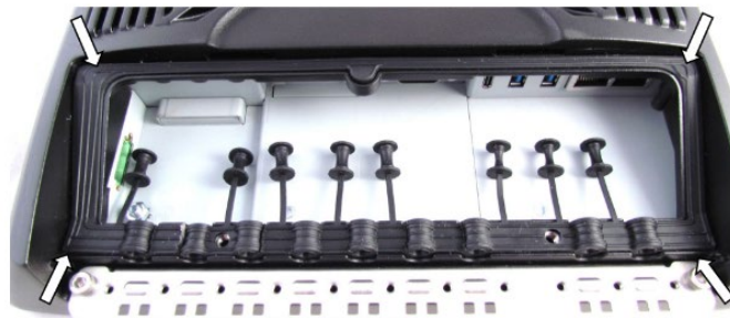
Fig. 14-4: Rubber seal inserted in the cable compartment
