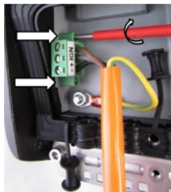
Fig. 14-9: Tighten power supply cable
