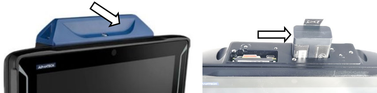
Fig. 8-1: Battery pocket with UPS DLT-V73A
