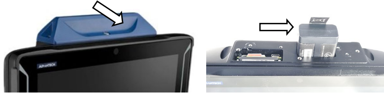
Fig. 2-1: Battery pocket with UPS DLT-V73A
