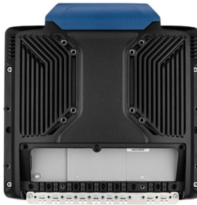
Fig. 13-1: VESA mounting hole pattern on the rear side of the DLT-V73A
