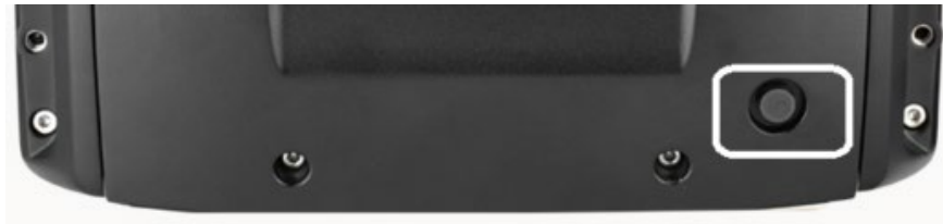
Fig. 14-15: Pressure compensation element
