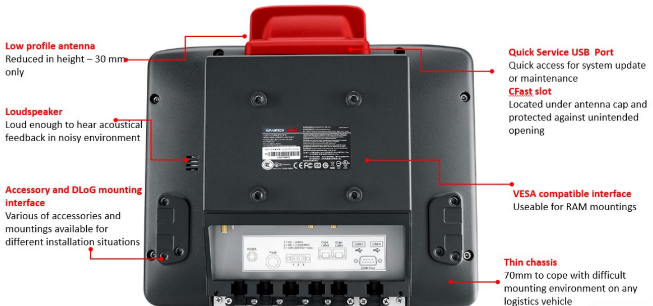
Fig. 2.2: Functional overview DLT-V6210FL back side
