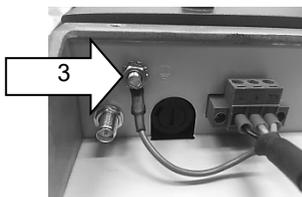
**NOTICE:** To make sure the device is grounding correctly, it is important to follow the correct order to put the components on the ground bolt as below (from inside to outside):
