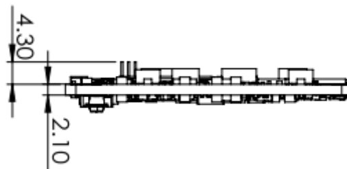
Figure 2.8 Pentium Series Board Mechanical Diagram – Side
