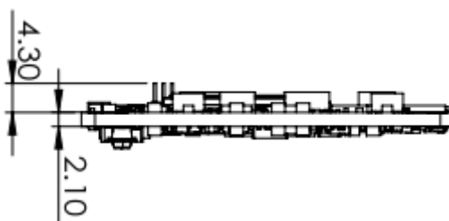
Figure 2.5 Atom Series Board Mechanical Diagram – Side
