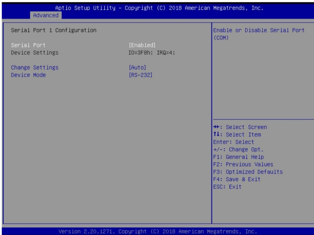
Figure 4.15 Serial Port 1 Configuration
