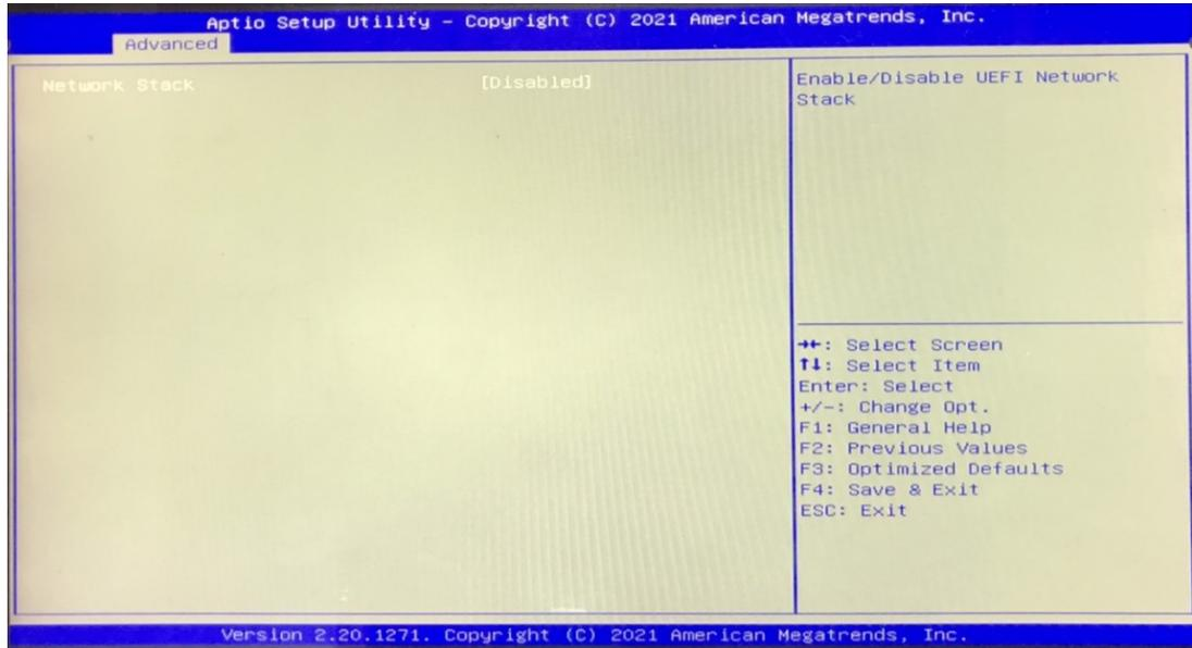
**Figure 4.23 Network Stack Configuration**
