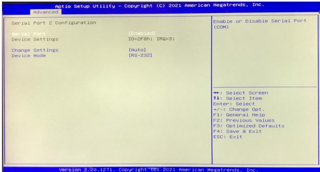
**Figure 4.17 Serial Port 2 Configuration**
