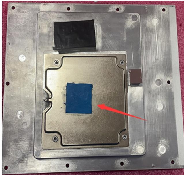
Figure 3.11 CPU thermal pad location
