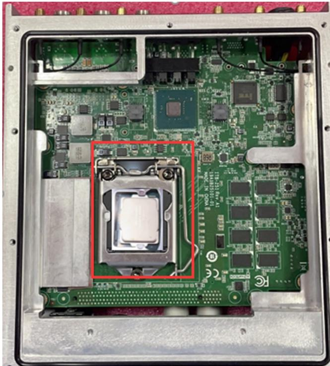
**Figure 3.12 CPU Socket**
