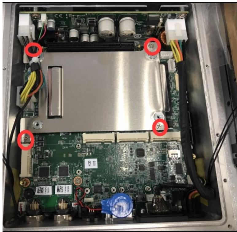
Figure 3.2 SSD Bracket screw locations
