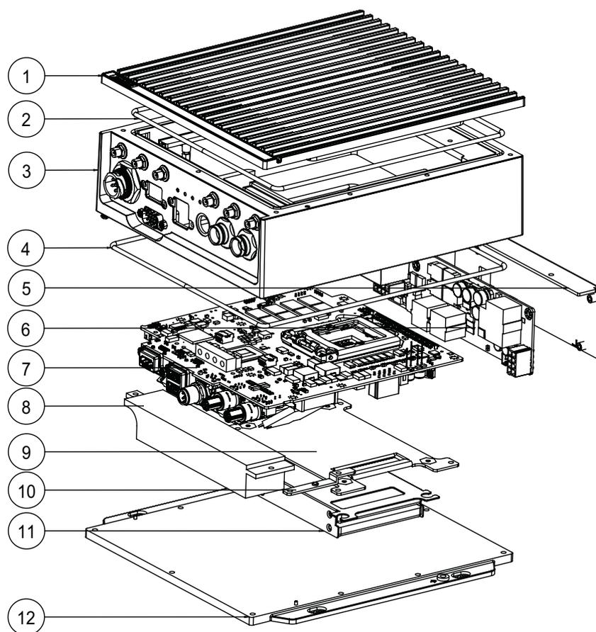
**Figure 1.2 ITA-460 Exploded Diagram**
