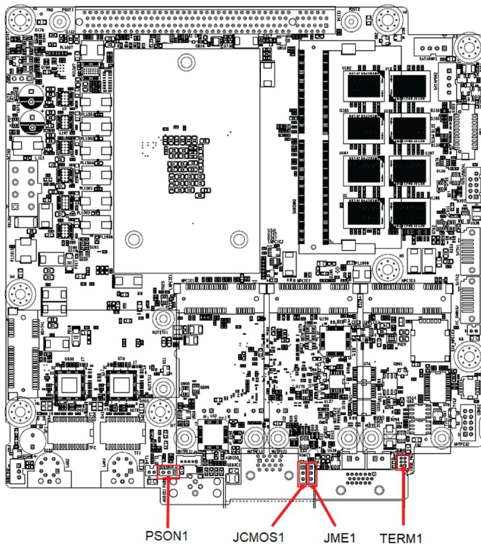
Figure 2.1 Jumper and Connector Locations on Main Board
