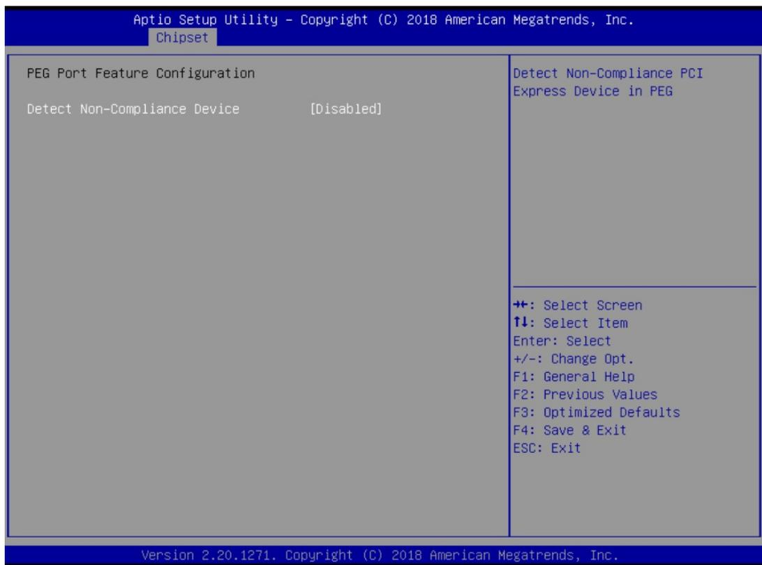
Figure 4.28 PEG Port Feature Configuration
