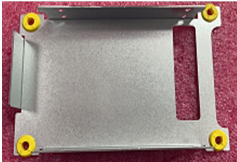
Figure 3.5 Dual-SSD Socket (2)
