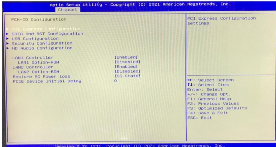
Figure 4.30 PCH-IO Configuration
