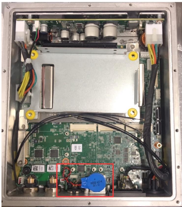
**Figure 3.13** RTC battery location
