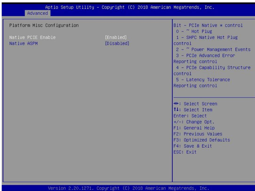
Figure 4.5 Platform Misc Configuration
