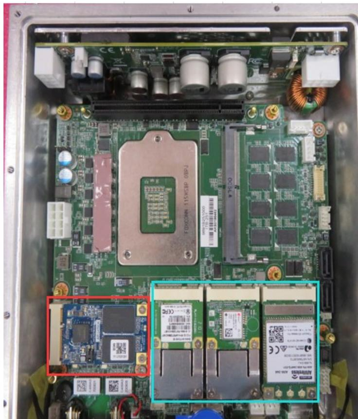
**Figure 3.3 Mini PCIe and mSATA Locations on Main Board**
