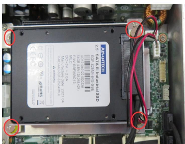
Figure 3.8 SSD socket screw locations
