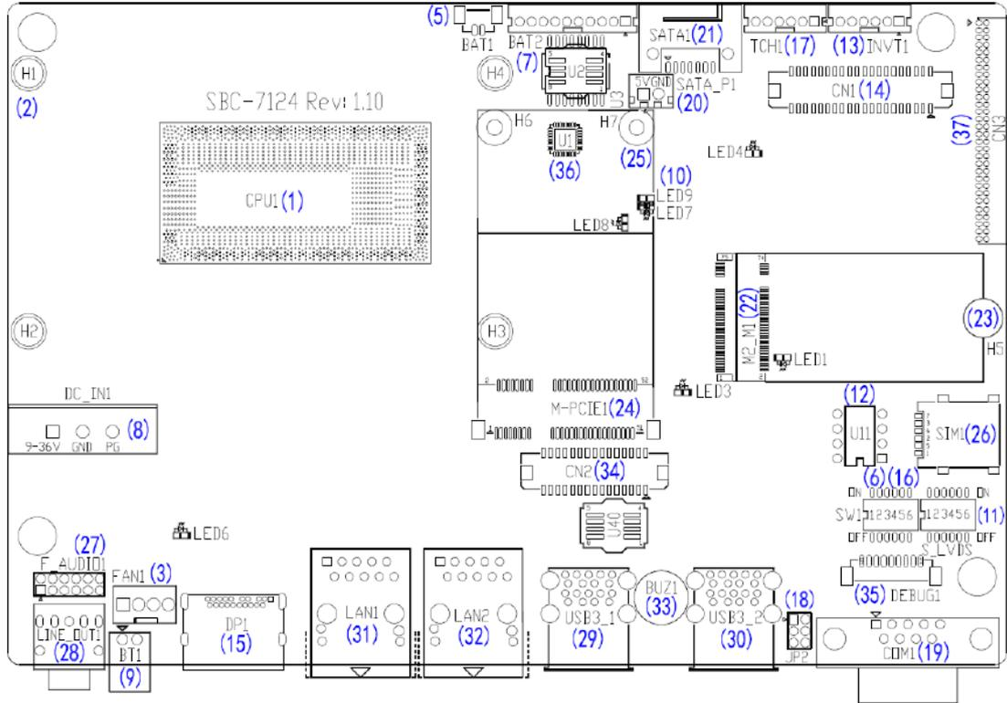
Figure 2.2: Jumpers and Connectors Location- Board Top
