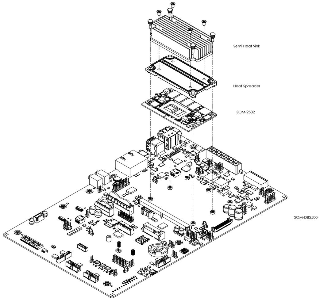
**Figure 2.10 Celeron® Pentium® (J and N Series) Board Assembly Drawing**
