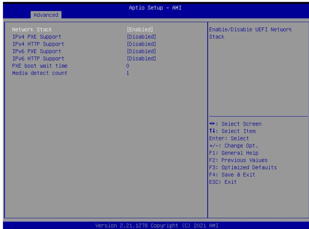
**Figure 3.17 Network Stack Configuration**
