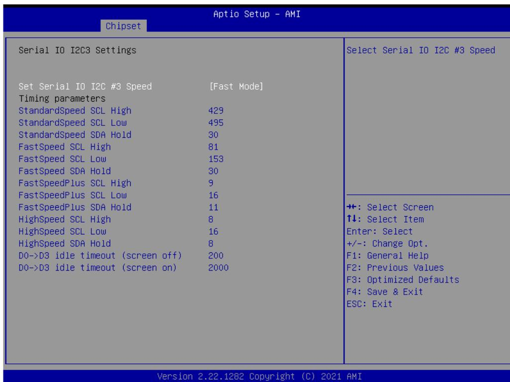
**Figure 3.38 Serial I/O I2C3 Settings**
