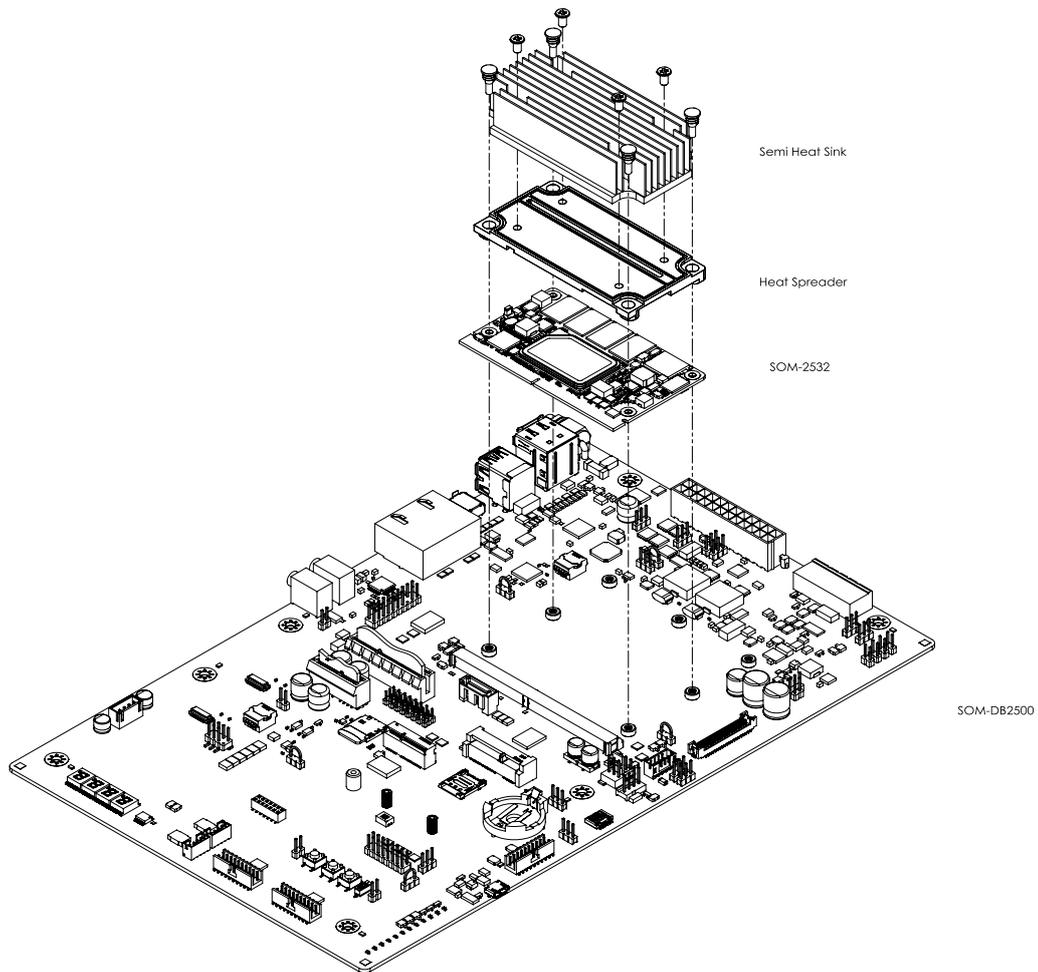
Figure 2.9 Atom® Series Assembly Drawing
