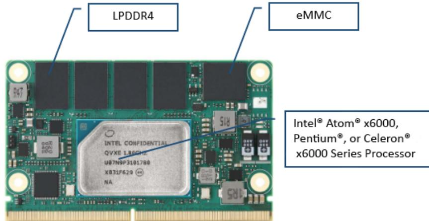
Figure 2.1 Board Chips ID — Front
