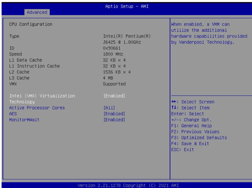
**Figure 3.4 CPU Configuration**
