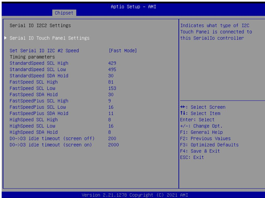
**Figure 3.37 Serial I/O I2C2 Settings**
