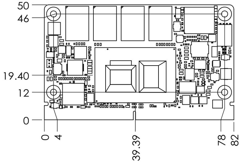
**Figure 2.6 Celeron® Pentium® (J and N Series) Board Mechanical Drawing - Front**
