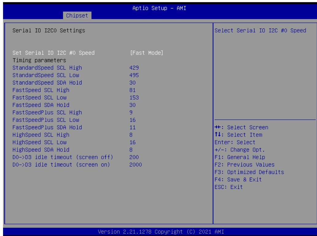
**Figure 3.36 Serial I/O I2C0 Settings**
