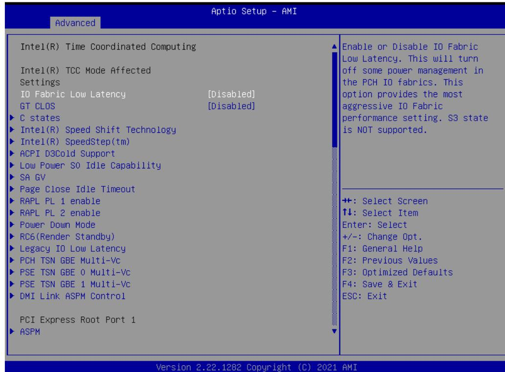
**Figure 3.7 Intel® Time Coordinated Computing**
