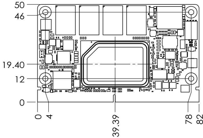
Figure 2.3 Atom® Series Board Mechanical Drawing - Front
