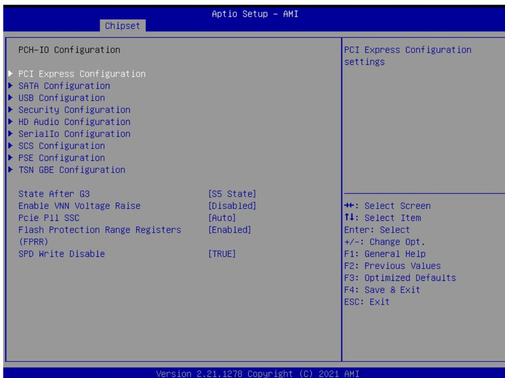
Figure 3.25 PCH-IO Configuration
