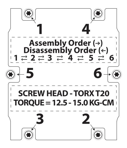
**WARNING:** Failure to attach thermal solutions one-at-a-time in the sequence 1-2-3-4-5-6 and failure to remove thermal solutions one at a time in the sequence 6-5-4-3-2-1 can lead to permanent socket damage.
