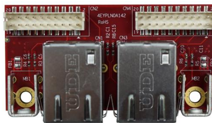
Figure 3: Mounting Hole Daughter Board Picture (EMPL-G201-C3/W3)
