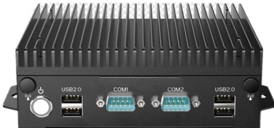
Figure 3.1-1 NBC-1360 panel diagram
