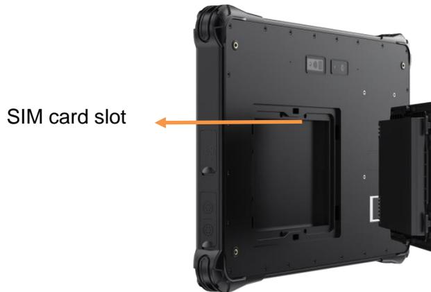
2. After installing the SIM card, you can connect to the 4G/5G network and surf the Internet normally.
