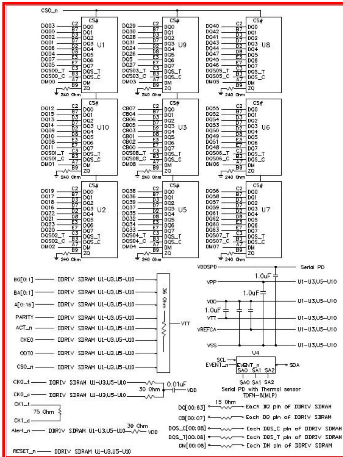
Note: 1. The ZQ ball on each DDR4 component is connected to an external  $240\Omega \pm 1\%$  resistor that is tied to ground. It is used for the calibration of the component's ODT and output driver.
