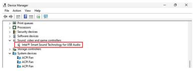
Note: After completing Intel<sup>®</sup> SST installation, the "Intel High Definition Audio" item will be shown at "Other devices" of Device Manager. Please install the audio codec driver for this.
