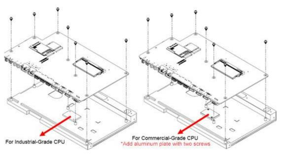
Disassemble the motherboard and heatsink by releasing the seven (7) screws shown above.
