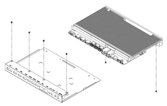
Separate the base and heatsink by releasing the six (6) screws shown above.
