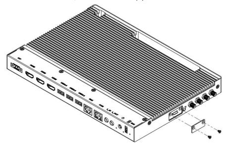
2. The following pictures show how to disassemble the system when replacing internal parts such as memory modules and M.2 cards.
