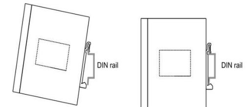
**STEP 2:** The DIN-Rail attachment unit will snap into place as shown below.
