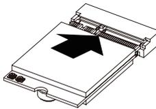
Step2. Secure it with the screw, tightening as necessary to fasten the M.2 WiFi module in place.
