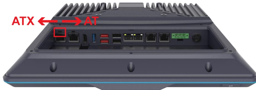
Figure 3-10: Power Switch Location
