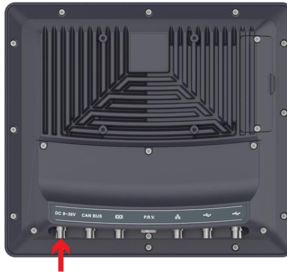
Figure 3-8: M12 Power Connector Location
