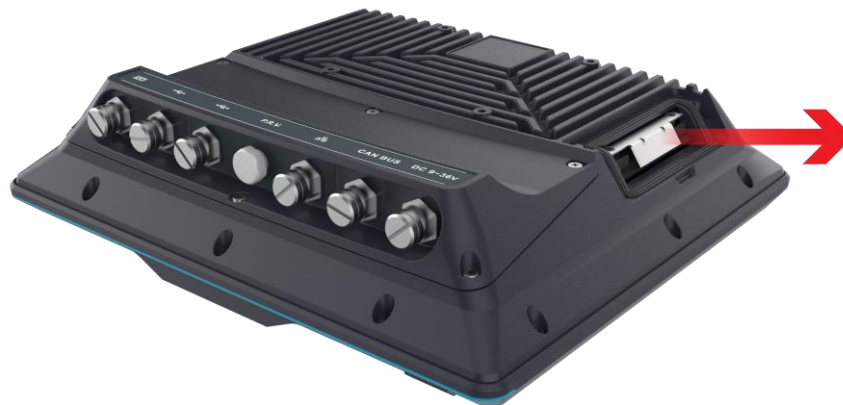
Figure 3-2: Remove SSD Bracket
